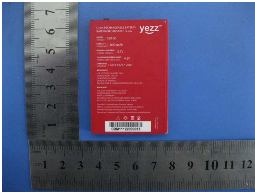
Battery - Top View
