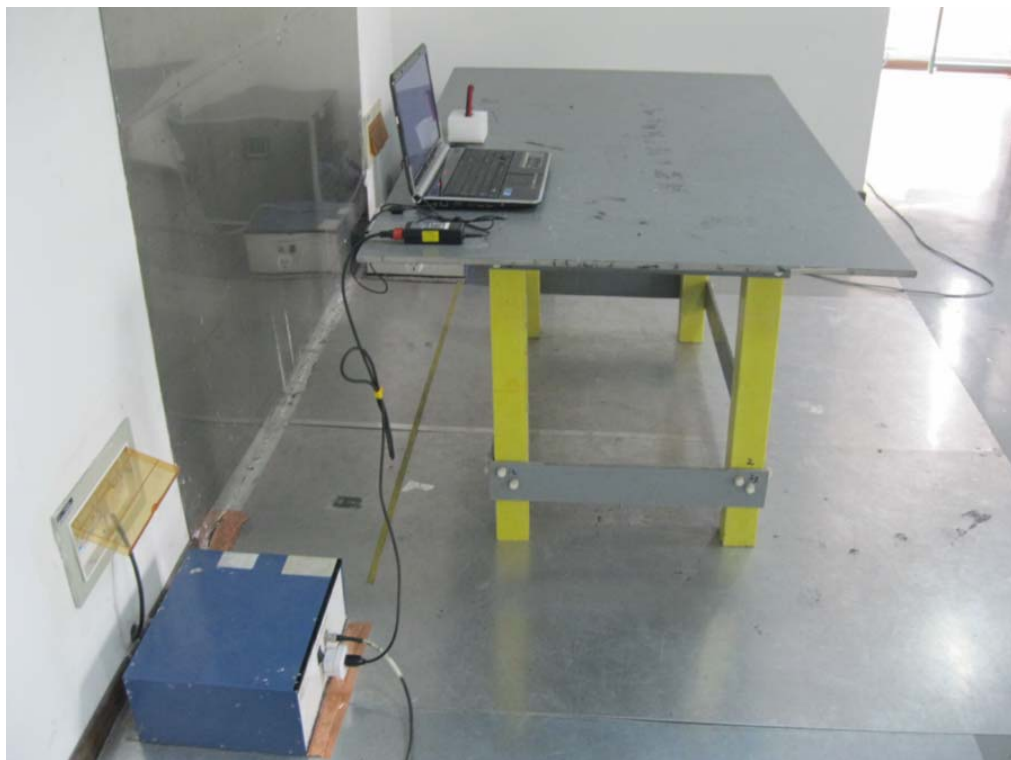
Conducted Emissions Test Setup - Side View
