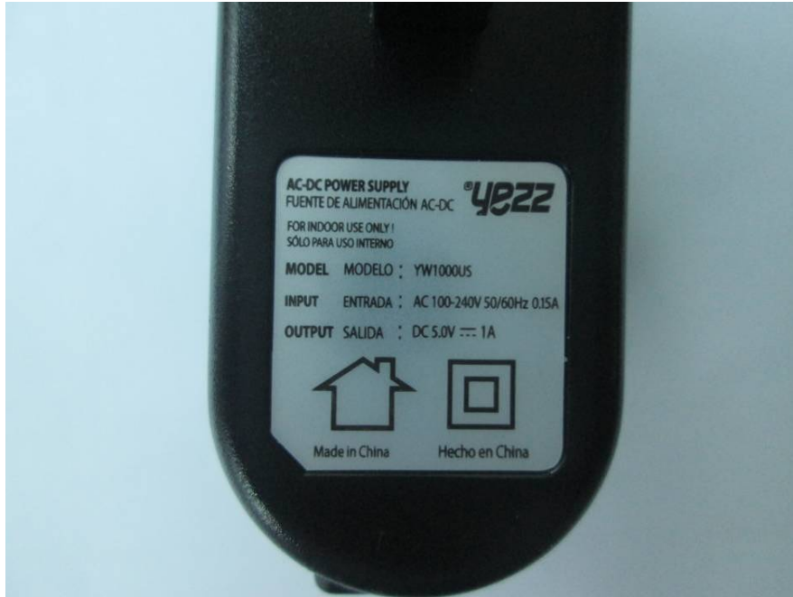
EUT – Adapter Label View
