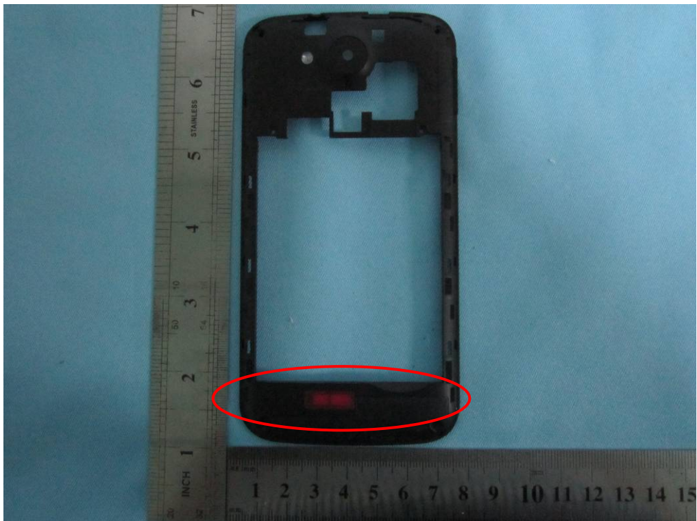
GSM / PCS/ UMTS Antenna View
