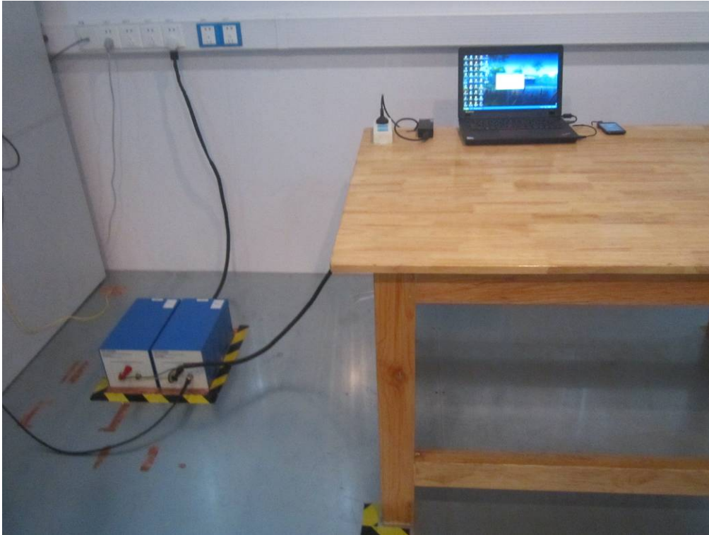
Conducted Emissions Test Setup Front View
