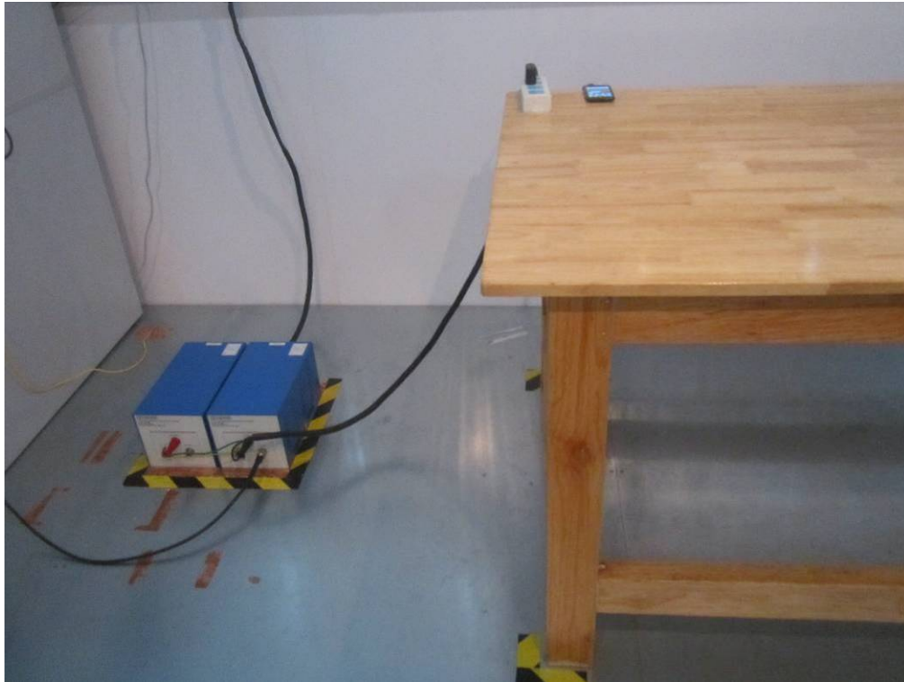
Conducted Emissions Test Setup Front View
