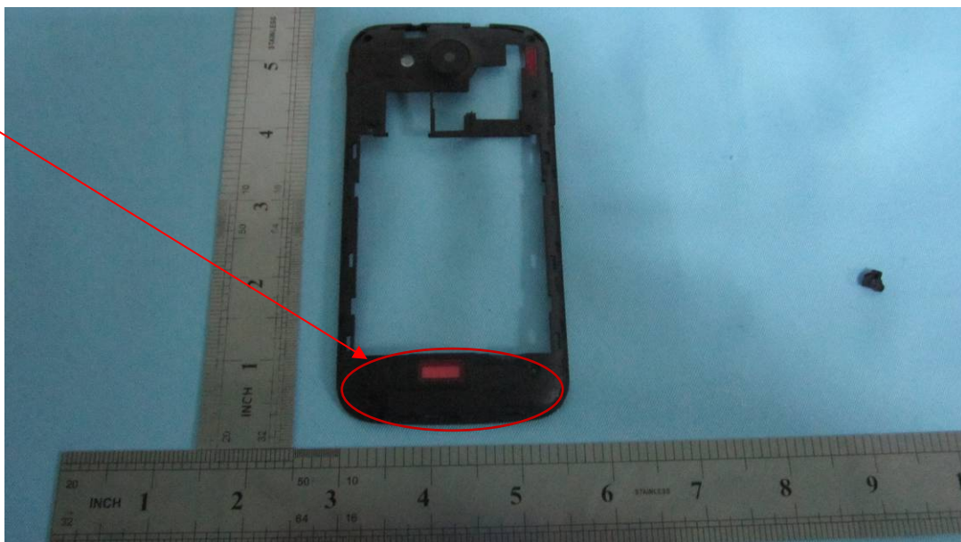
GSM / PCS/ UMTS Antenna View
