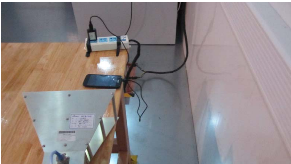
Conducted Emissions Test Setup Side View
