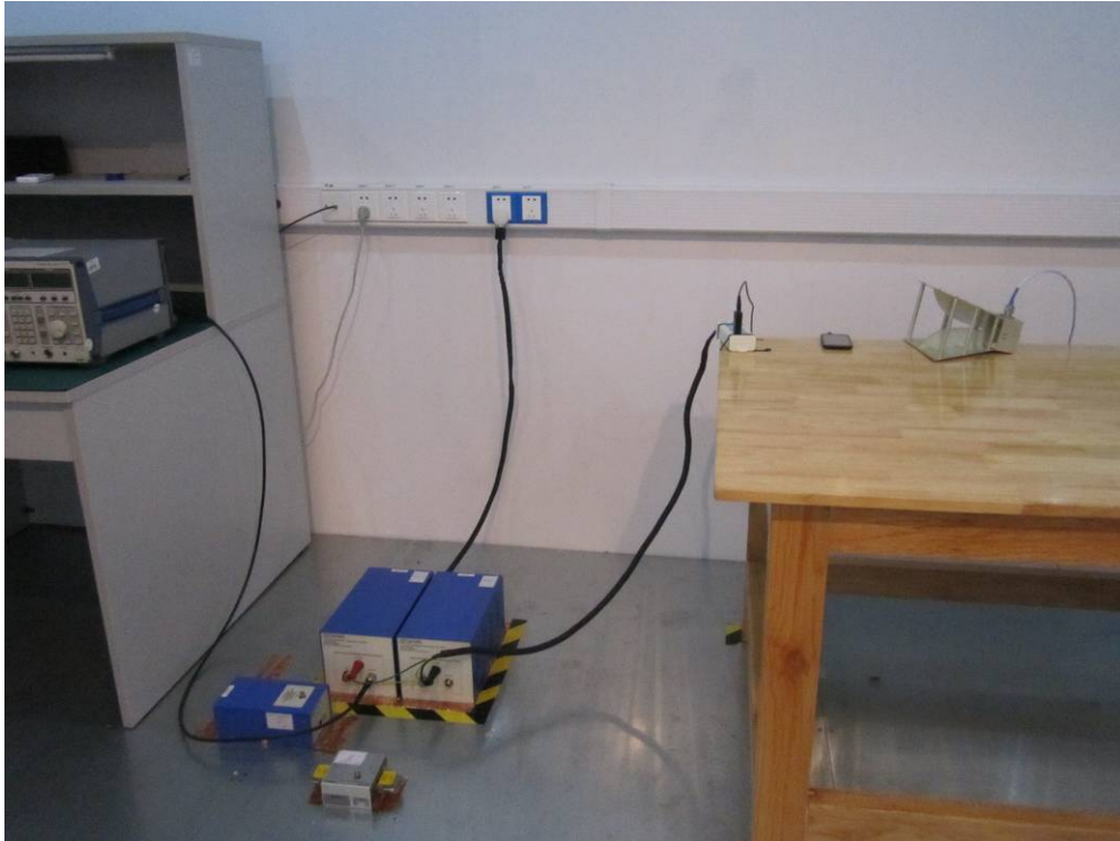
Conducted Emissions Test Setup Front View
