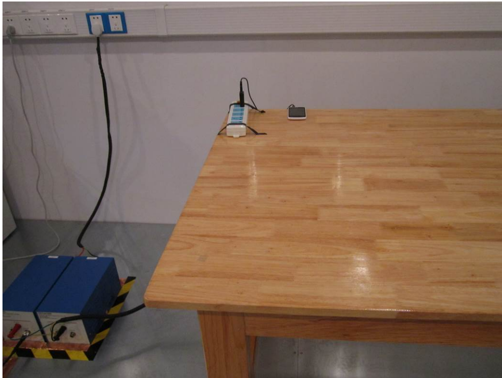
Conducted Emissions Test Setup Front View
