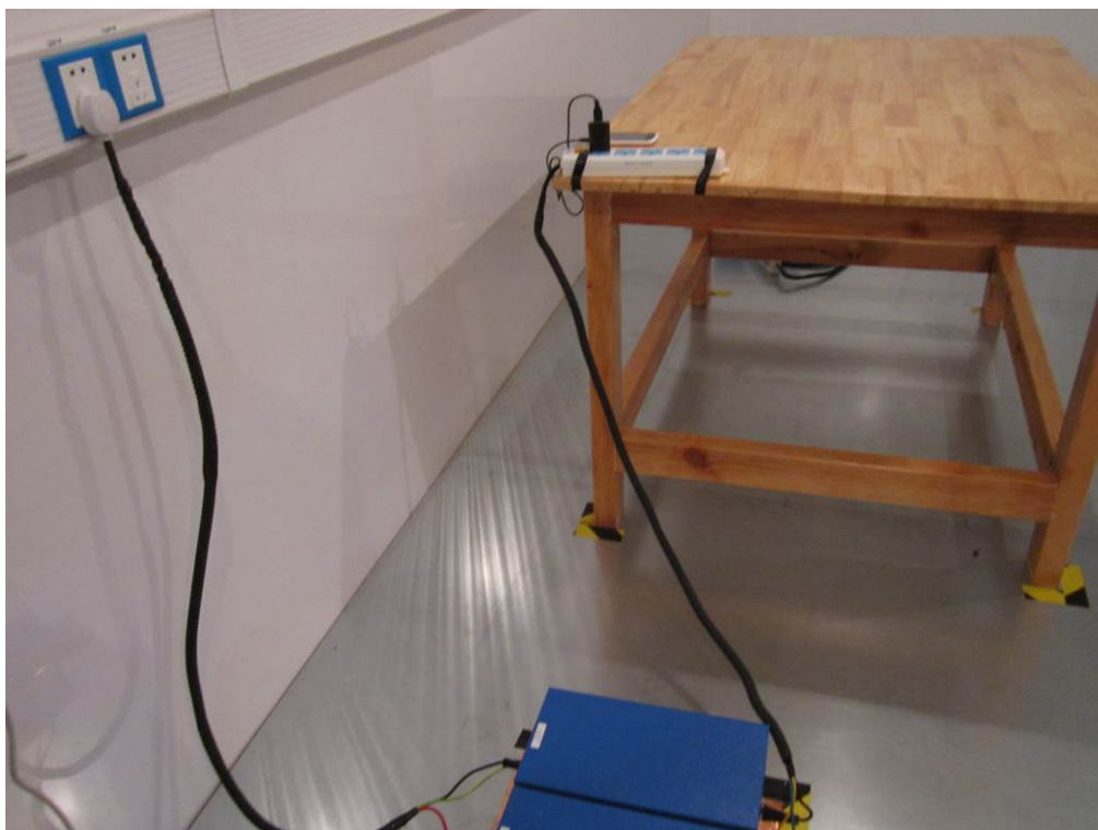
Conducted Emissions Test Setup Side View
