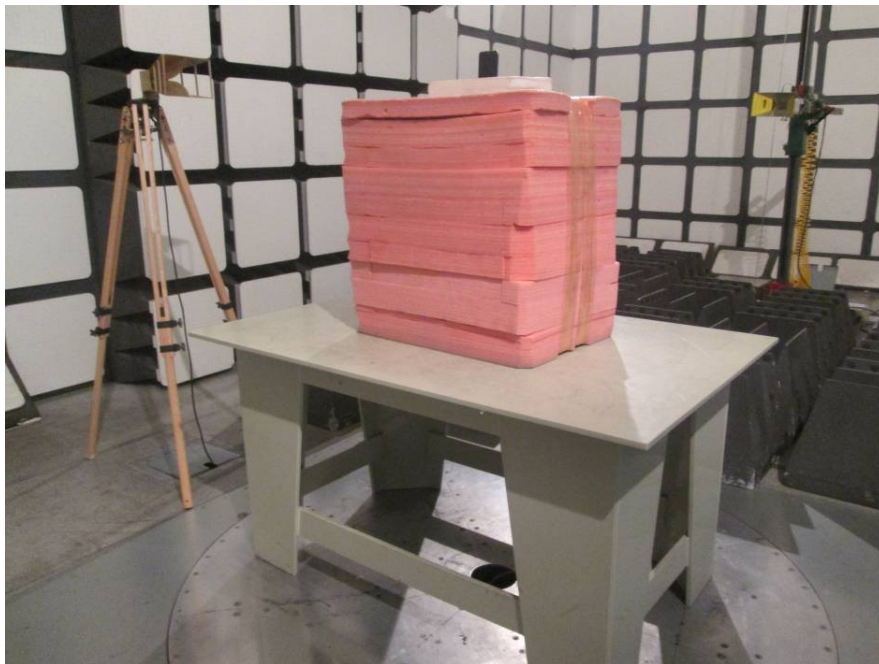
Radiated Emissions Test View (Above 1 GHz)
