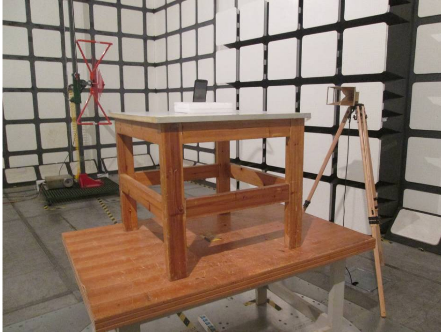
Radiated Emissions Test View (Below 1 GHz)
