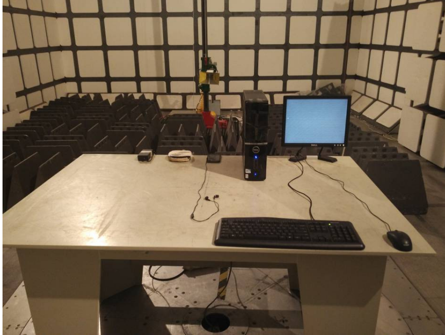
Radiated Emissions – Front View (Above 1 GHz)
