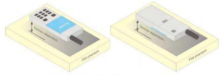
Figure 5 - Test positions for body-worn devices
