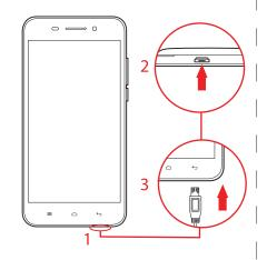
EN Insert USB cable and charge for 8 hours
