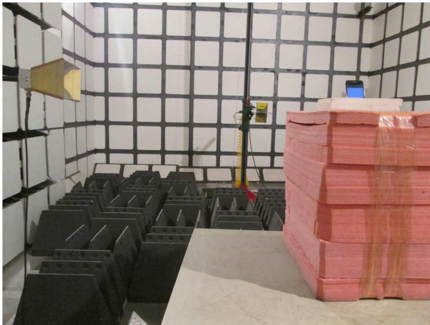
Radiated Emissions Test View (Above 1 GHz)
