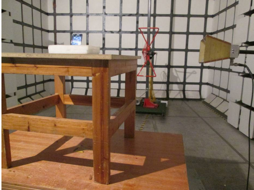
Radiated Emissions Test View (Below 1 GHz)
