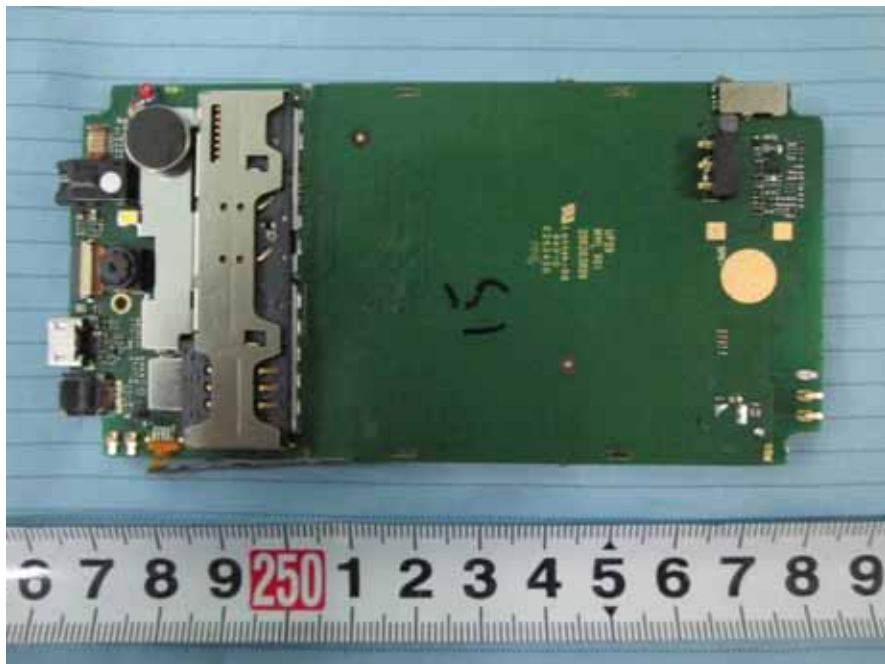
EUT – Main Board Bottom View
