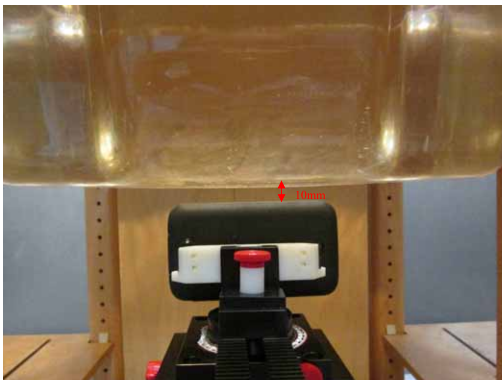
Body-worn Right Setup Photo (10mm)
