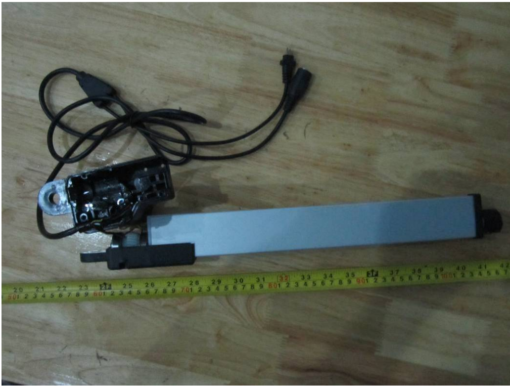
Lift Actuator- Uncover View
