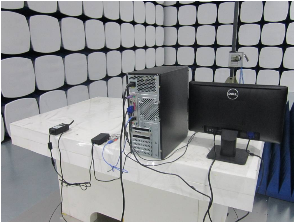
Radiated Spurious Emissions Test Setup Above 1GHz –Front View
