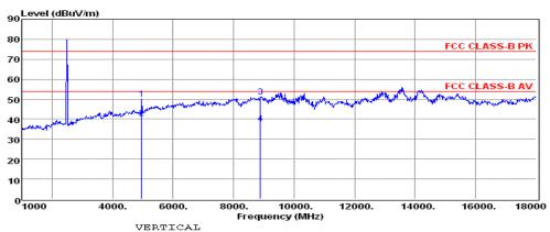
pol: Reading CabLos Antfac Measured Limit Over Freq Remark MHzdBuV dВ dB/m dBuV/m dBuV/m dВ 4960.00 45.27 7.78 50.35 74.00 -23.65 Peak 7.78 9.78 9.78 33.70 37.67 37.67 4960.00 35.25 40.33 54.00 -13.67 Average 3 4 8888.00 39.45 51.18 74.00 -22.82 Peak -16.34 8888.00 25.93 37.66 54.00
