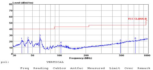
dB/m dBuV dВ dBuV/m dBuV/m MHz dB. 8.29 0.38 13.02 37.81 21.69 40.00 -18.31 QP 9.15 13.55 23.11 -16.89 44.28 0.41 40.00 QP 3 60.70 14.13 0.49 12.41 27.03 40.00 -12.97 QP 4 104.54 2.08 0.61 12.75 15.44 43.50 -28.06 QP 5 492.47 0.73 1.50 16.39 18.62 46.00 -27.38 QP 1.55 1.70 6 726.81 19.15 22.40 46.00 -23.60 OP
