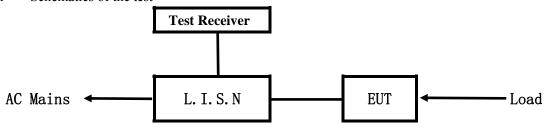
**EUT**: Equipment Under Test
