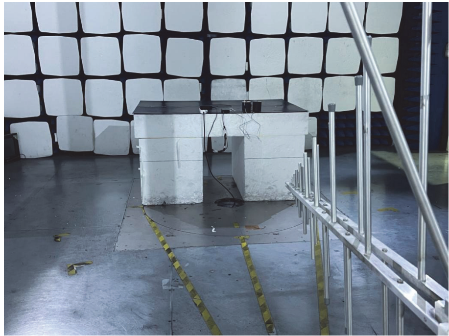
Radiation Emission Test Setup (30MHz to 1GHz)
