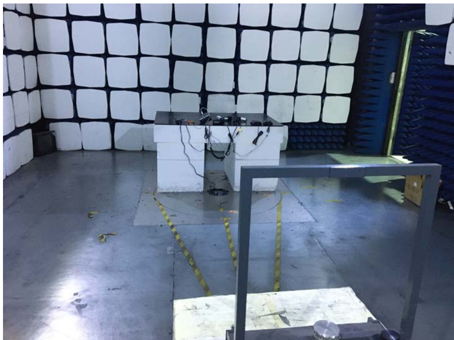
Radiation Emission Test Setup (Below 30MHz)
