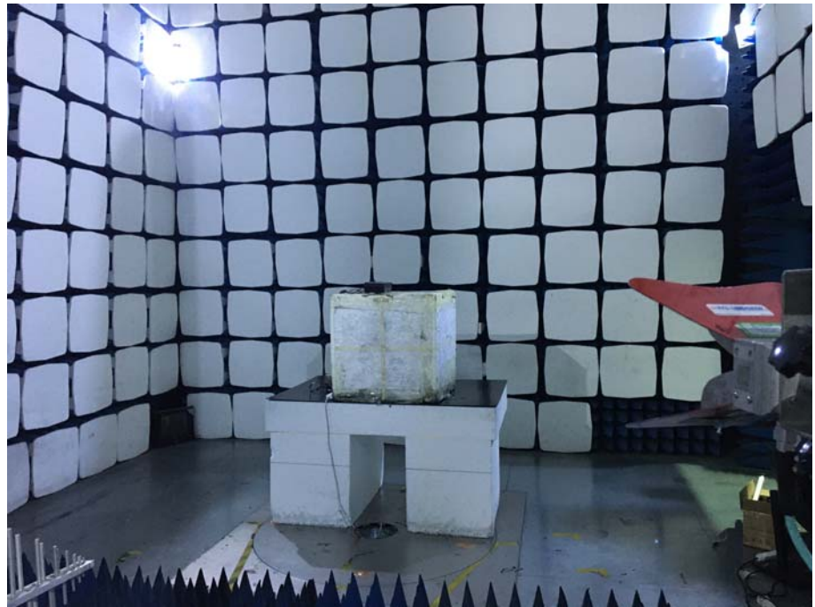
Radiation Emission Test Setup (1GHz to 18GHz)
