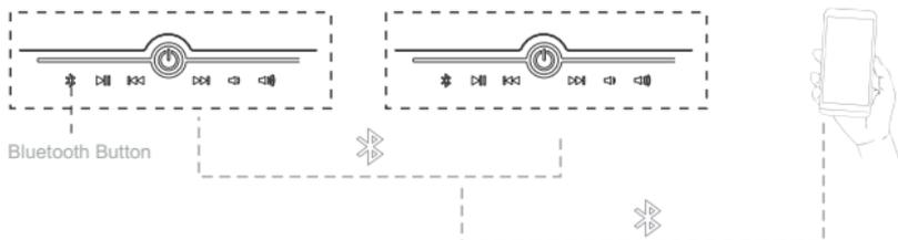
Touch and hold both Bluetooth Buttons for 3 seconds, the indicators become flashing slowly, then the iTable minis will connect to each other automatically.
