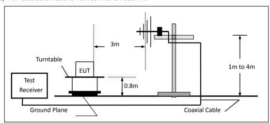
(c) For radiated emissions above 1000MHz
