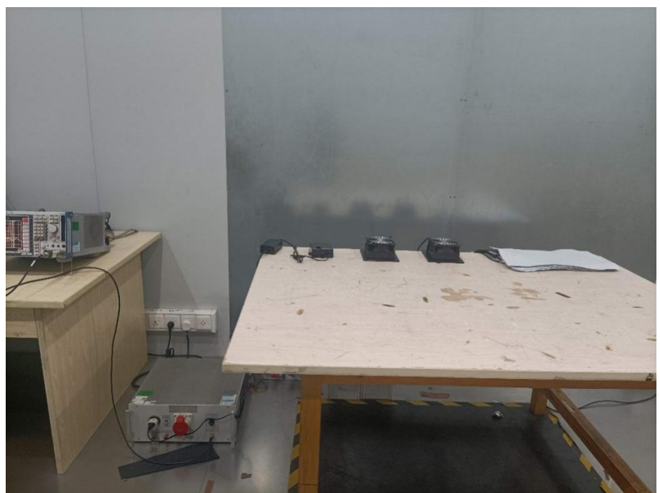
Conducted Emission Test Setup
