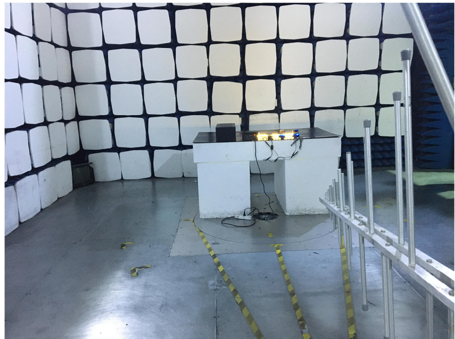
Radiation Emission Test Setup (30MHz to 1GHz)
