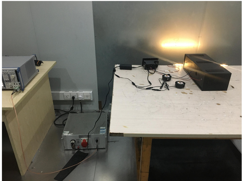
Conducted Emission Test Setup
