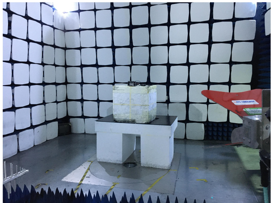
Radiation Emission Test Setup (1GHz to 18GHz)
