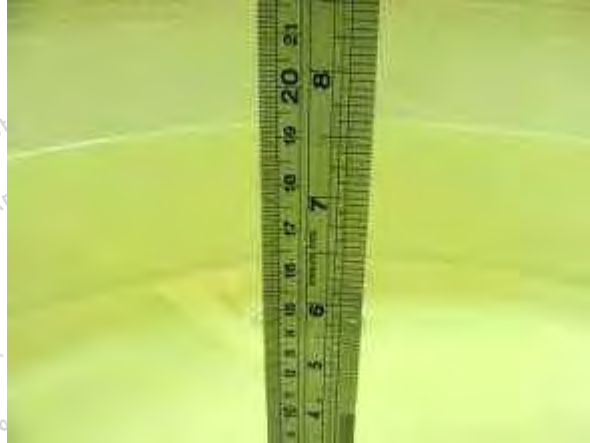
Photo of Liquid Height for Head SAR
