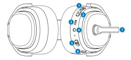
The mic boom arm, ports, LEDs, and function buttons on the ClearDryve® headphone are on the same earpiece. You can use this earpiece on either ear. ClearDryve® automatically adjusts for either side when you extend the mic arm. To switch the earpiece with controls from one ear to the other, swivel the mic boom up and over to the other side.
