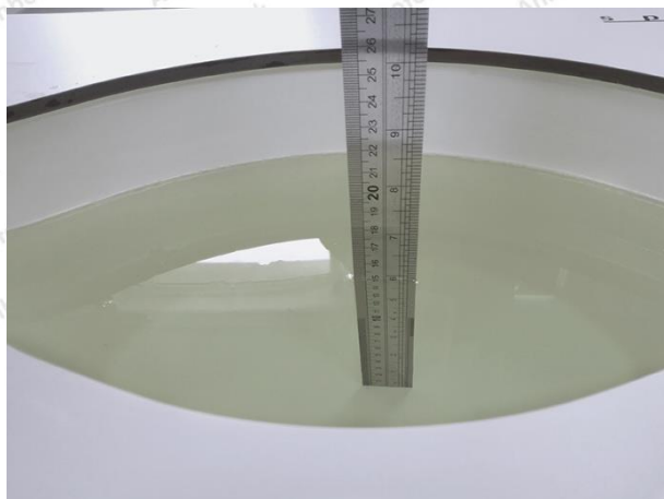
Liquid depth in the body phantom (2450MHz)
