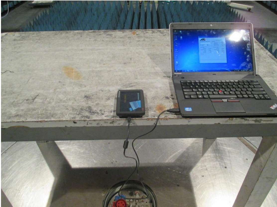
Conducted Emission Test setup photo
