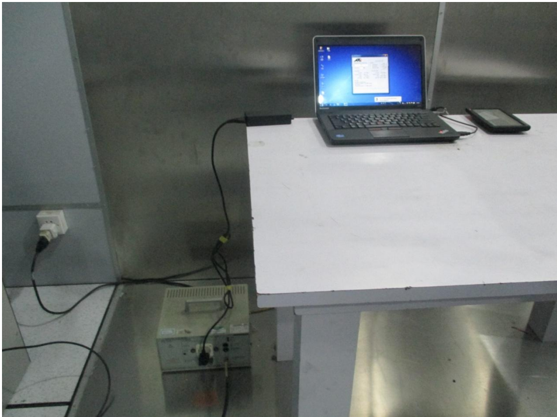
Conducted Emission Test setup photo
