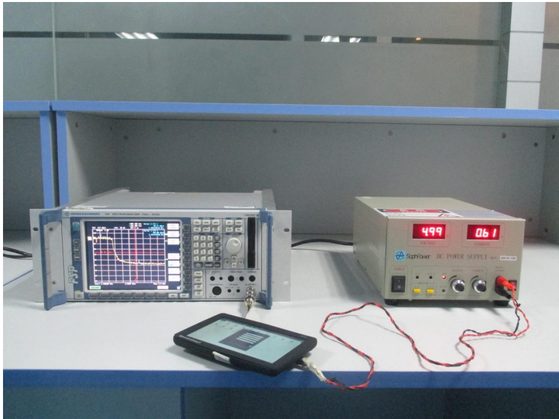
Conducted Test setup photo
