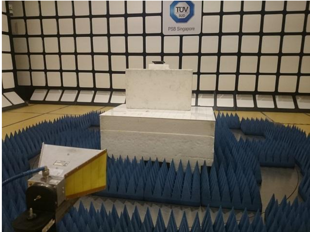
Radiated Emissions Test Setup (Front View)
