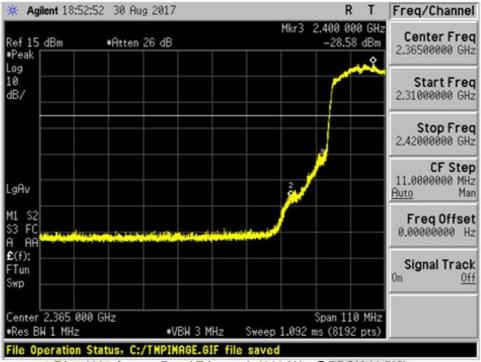
Plot 428 - Lower Band Edge at 2.4000GHz @BPSK 13.5Mbps
