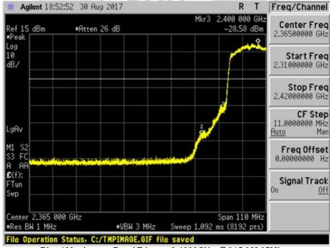
Plot 423 – Lower Band Edge at 2.4000GHz @64QAM 65Mbps
