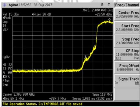
Plot 431 – Lower Band Edge at 2.4000GHz @64QAM 135Mbps
