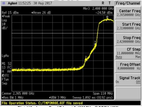
Plot 413 – Lower Band Edge at 2.4000GHz @QPSK 18Mbps
