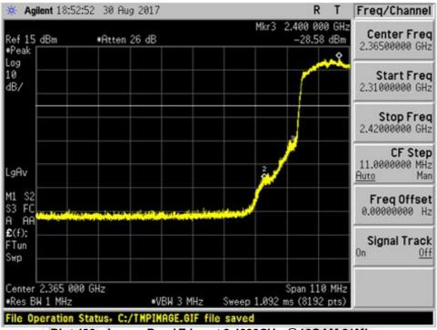
Plot 430 - Lower Band Edge at 2.4000GHz @16QAM 81Mbps
