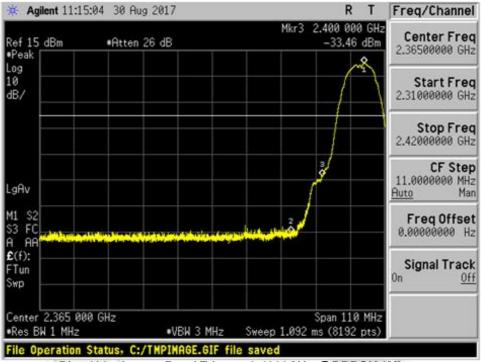
Plot 406 - Lower Band Edge at 2.4000GHz @DBPSK 1Mbps
