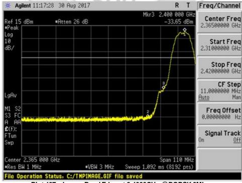
Plot 407 - Lower Band Edge at 2.4000GHz @DQPSK 2Mbps
