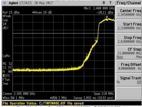
Plot 421 – Lower Band Edge at 2.4000GHz @QPSK 19.5Mbps
