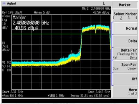
Plot 444 - Peak Plot at Lower Band Edge at 2.4000GHz
