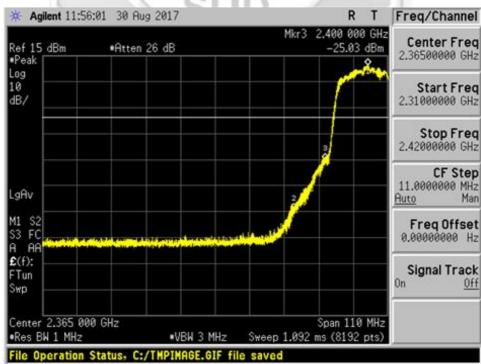
Plot 415 - Lower Band Edge at 2.4000GHz @64QAM 54Mbps
