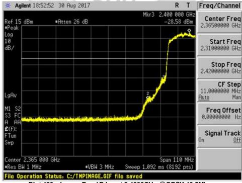
Plot 429 - Lower Band Edge at 2.4000GHz @QPSK 40.5Mbps
