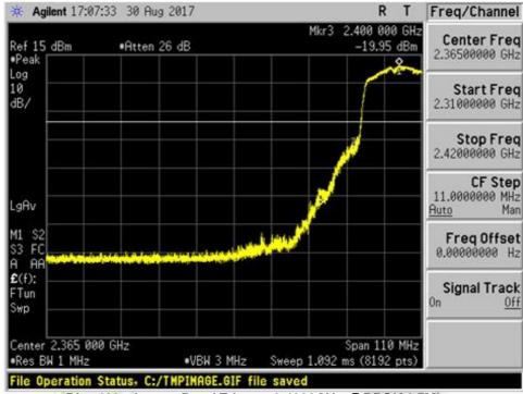
Plot 420 - Lower Band Edge at 2.4000GHz @BPSK 6.5Mbps
