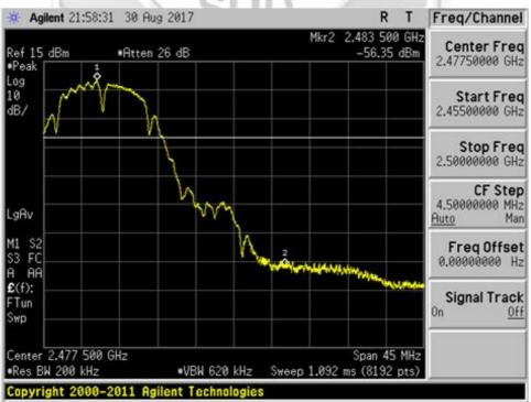
Plot 410 – Upper Band Edge at 2.4835GHz @DQPSK 2Mbps
