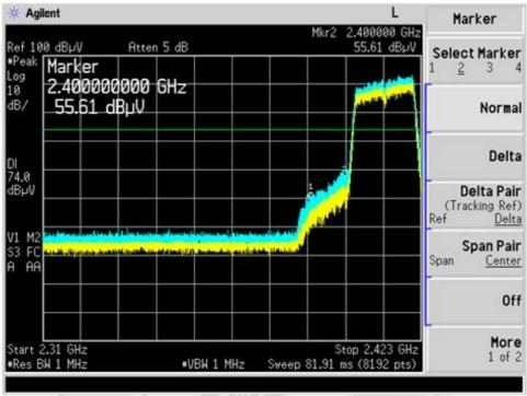
Plot 438 - Peak Plot at Lower Band Edge at 2.4000GHz
