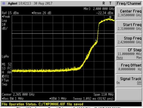
Plot 422 - Lower Band Edge at 2.4000GHz @16QAM 39Mbps
