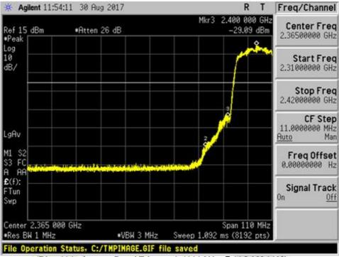
Plot 414 - Lower Band Edge at 2.4000GHz @16QAM 36Mbps
