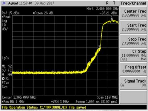
Plot 412 - Lower Band Edge at 2.4000GHz @BPSK 9Mbps
