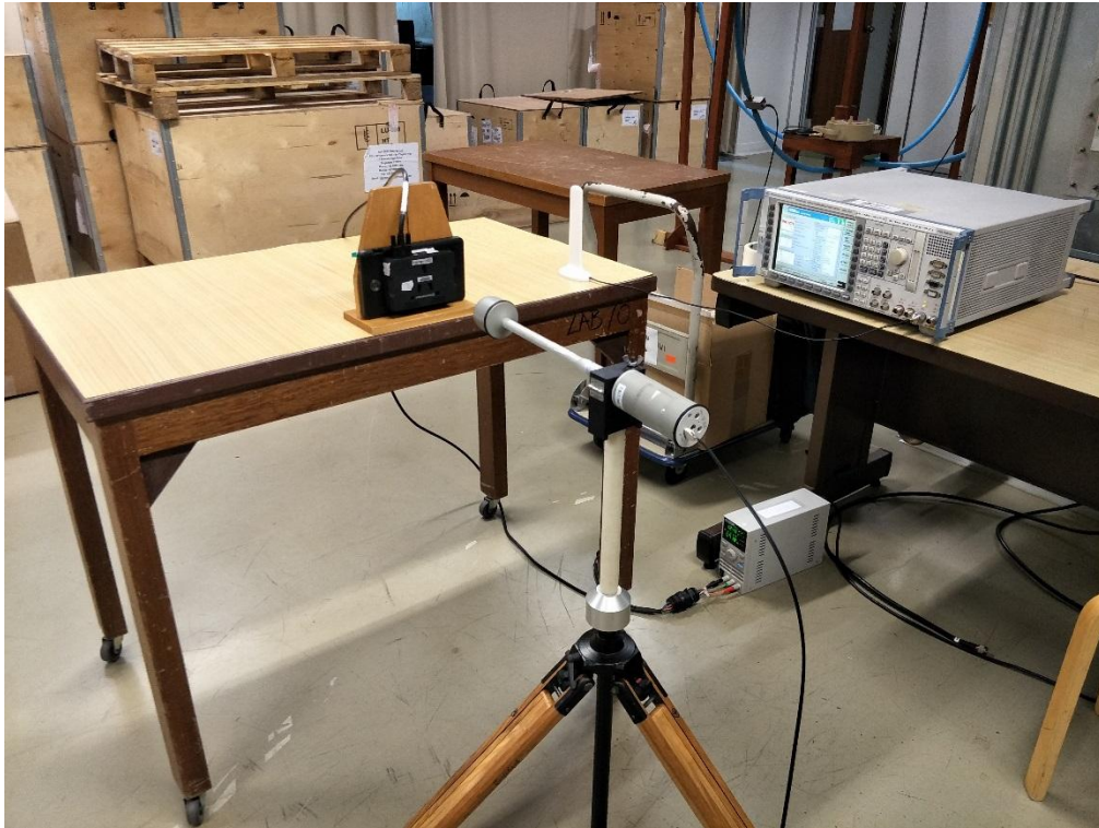
Maximum Permissible Exposure (MPE) Test Setup
