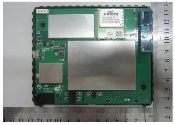
2. Mainboard rear view with shielding
