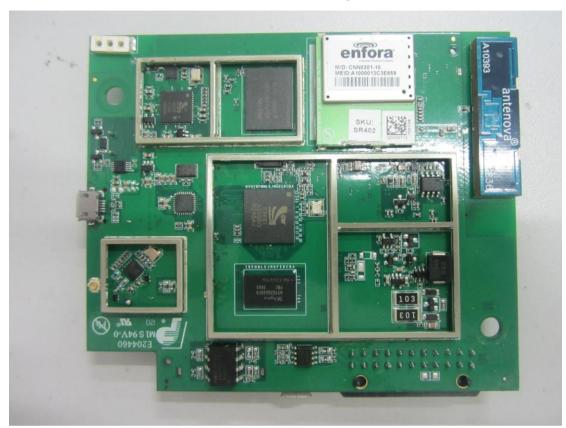
3. Mainboard front view without shielding
