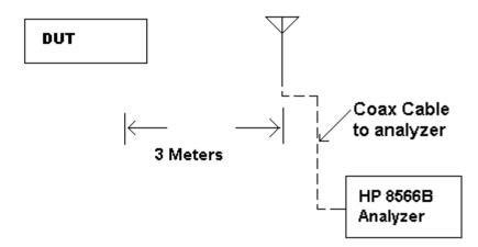
METHOD OF MEASUREMENT: The procedure used was ANSI standard C63.4-2003 & the FCC/OET Guidance on Measurements for Spread Spectrum Systems – KDB 558074 dated March 23, 2005.
