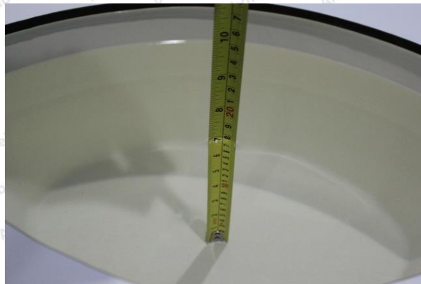
Liquid depth in the body phantom (5GHz)
