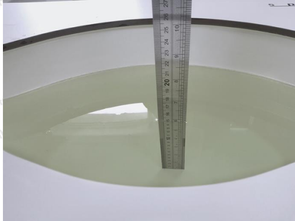
Liquid depth in the body phantom (2450MHz)
