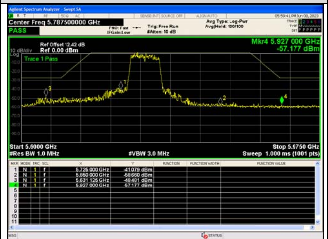
Out Of Band Emission IEEE 802.11ac_Channel 151_40MHz_Antenna 0
