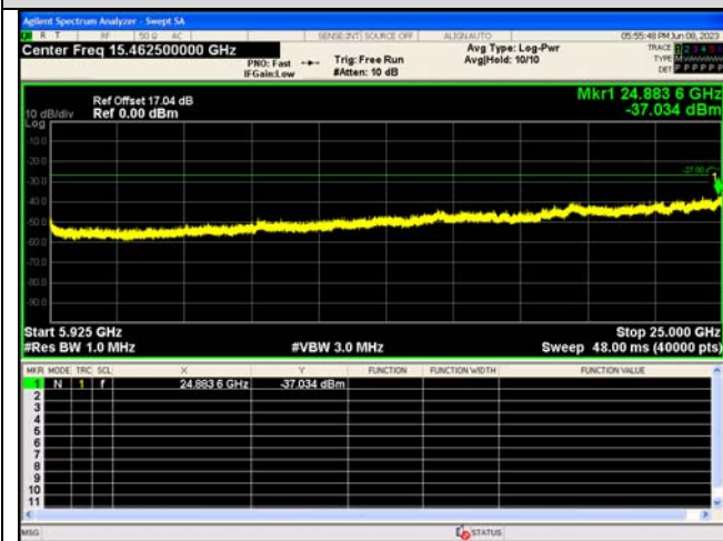
Spurious Emission:5925~25000.0 MHz IEEE 802.11ac_Channel 165_20MHz_Antenna 0
