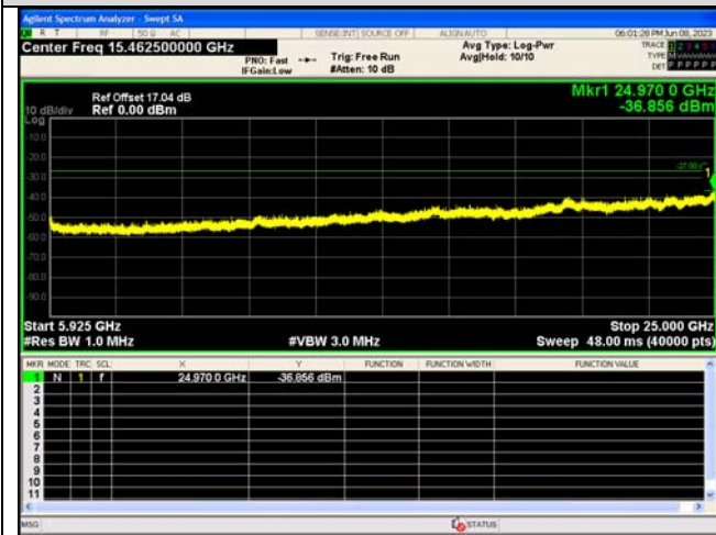
Spurious Emission:5925~25000.0 MHz IEEE 802.11ac_Channel 159_40MHz_Antenna 0
