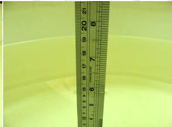
Photo of Liquid Height for Body SAR
