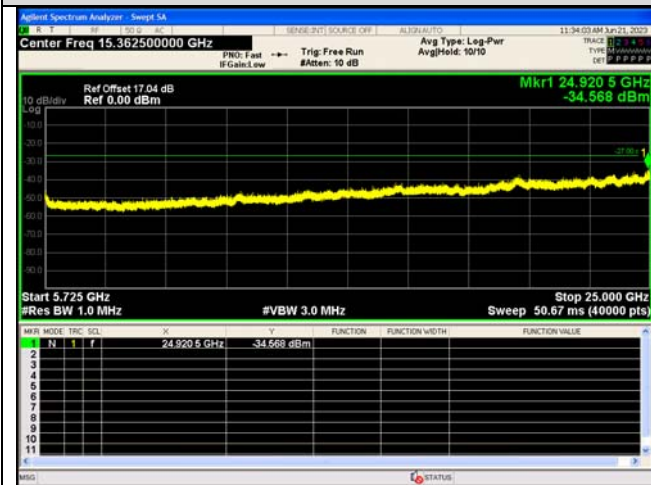
Spurious Emission:5725~25000.0 MHz IEEE 802.11a_Channel 100_20MHz_Antenna 0
