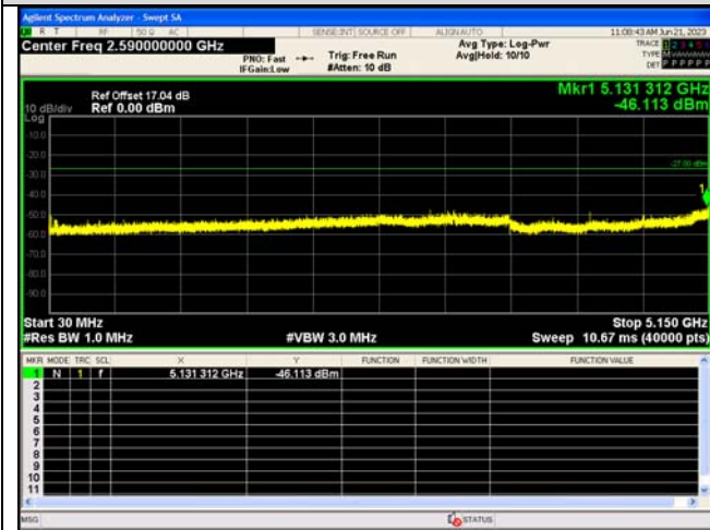
Spurious Emission:30.0~5150 MHz IEEE 802.11n_Channel 56_20MHz_Antenna 0
