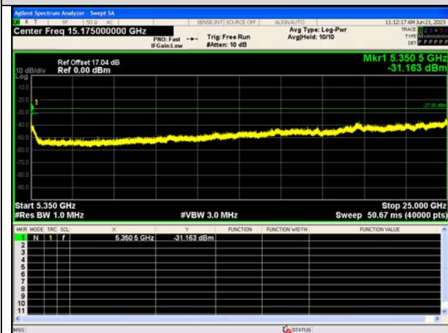
Spurious Emission:5350~25000.0 MHz IEEE 802.11n_Channel 64_20MHz_Antenna 0
