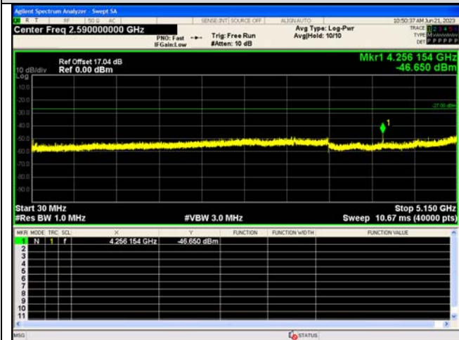
Spurious Emission:30.0~5150 MHz IEEE 802.11a_Channel 64_20MHz_Antenna 0
