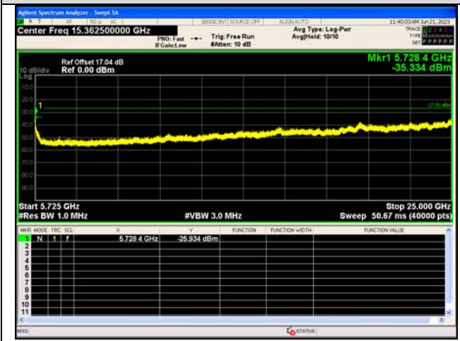
Spurious Emission:5725~25000.0 MHz IEEE 802.11a_Channel 140_20MHz_Antenna 0
