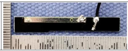
The antenna is PCB antenna with ipex connector. The best case gain of the antenna is 0dBi.
