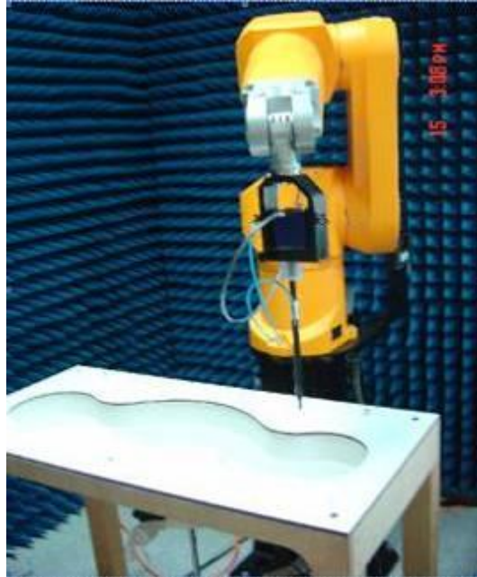
Photo 1: SAR measurement System
