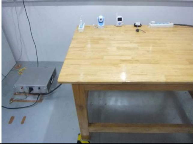
Conducted Emissions Test Setup – 433MHz Front View
