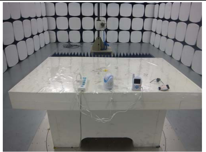
Radiated Emissions Test Setup Above 1GHz – 433MHz Side View
