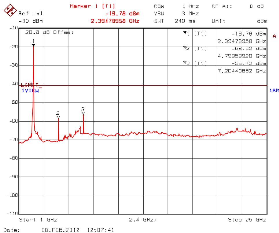
**Plot 5.9.4.3.17. Spurious RF Conducted Emissions into Restricted Bands, Transceiver 2**
