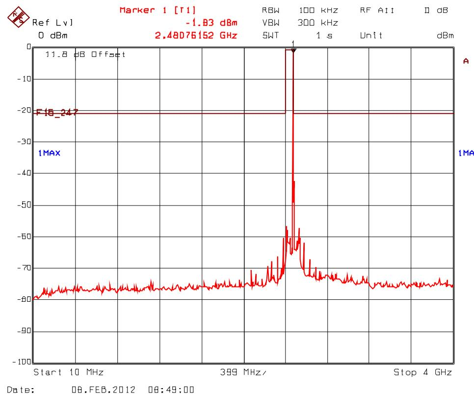
**Plot 5.9.4.2.12.** Spurious RF Conducted Emissions into Non-Restricted Bands, Transceiver 2
