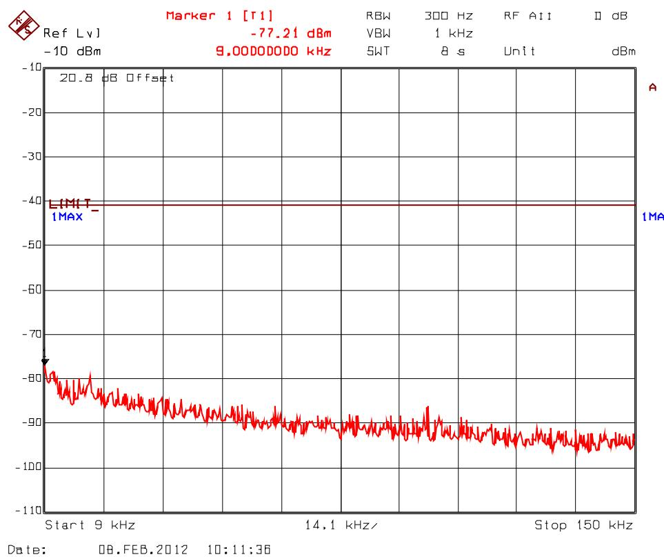
**Plot 5.9.4.3.22. Spurious RF Conducted Emissions into Restricted Bands, Transceiver 2
