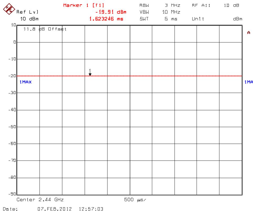
**Plot 5.8.4.9.** Maximum Peak Conducted Output Power, Low Power Setting
