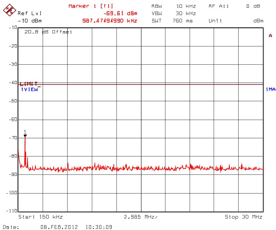
**Plot 5.9.4.3.3. Spurious RF Conducted Emissions into Restricted Bands, Transceiver 1**
