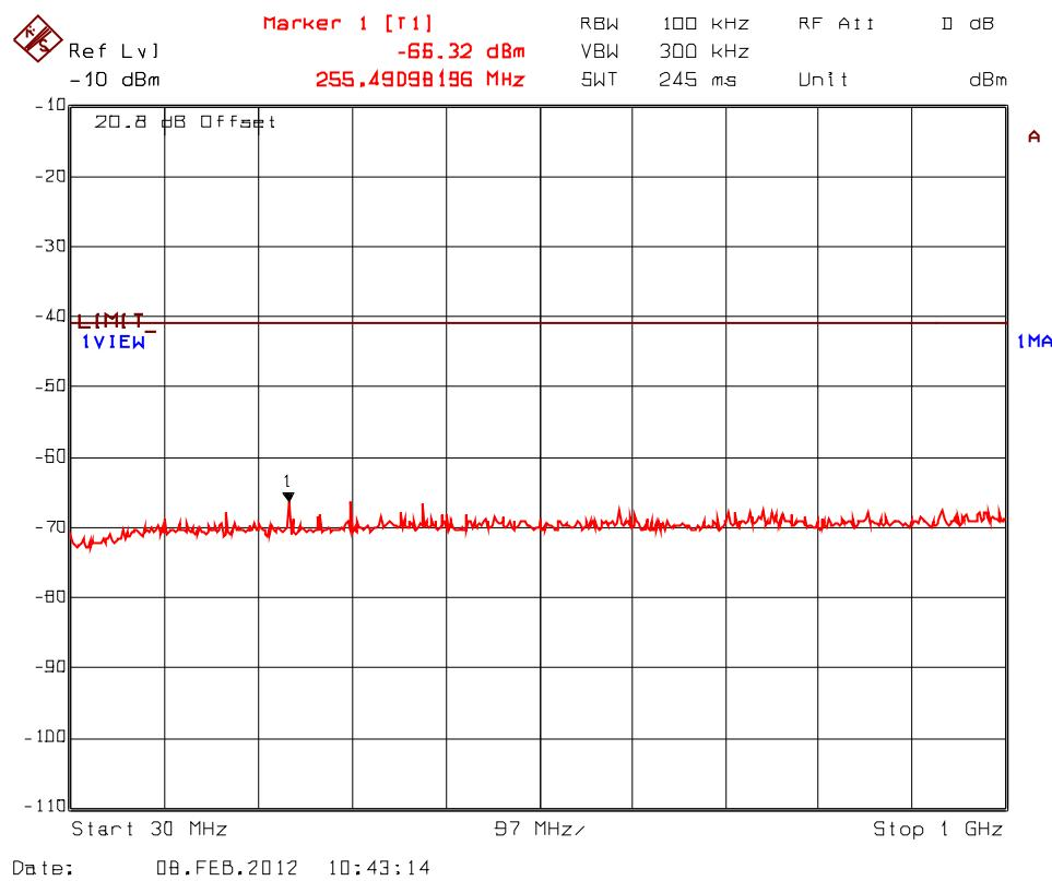
**Plot 5.9.4.3.16.** Spurious RF Conducted Emissions into Restricted Bands, Transceiver 2
