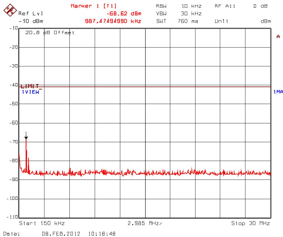
**Plot 5.9.4.3.15.** Spurious RF Conducted Emissions into Restricted Bands, Transceiver 2
