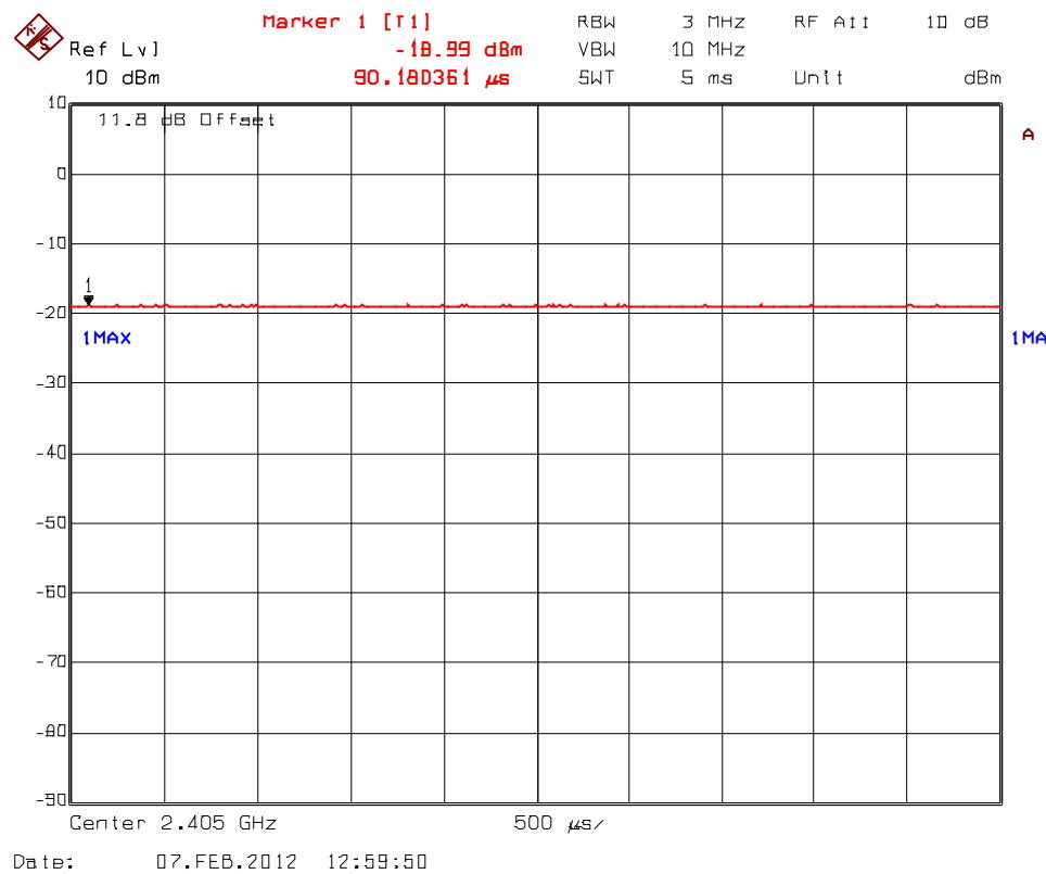
**Plot 5.8.4.11. Maximum Peak Conducted Output Power, Low Power Setting**
