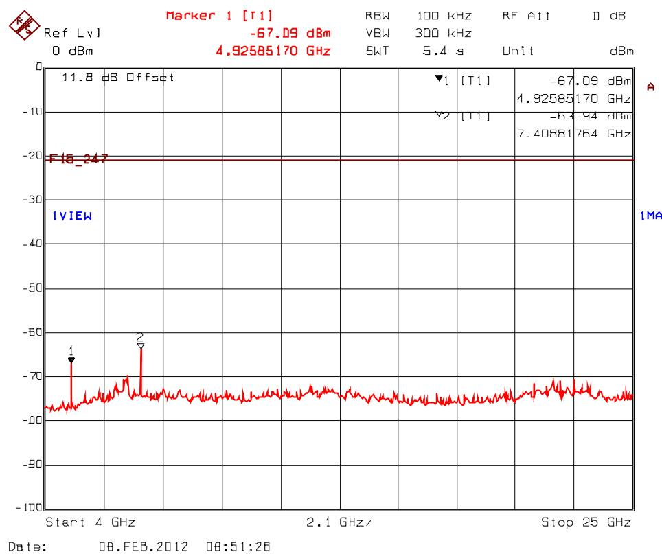
5.9.4.3. Spurious RF Conducted Emissions into Restricted Frequency Bands (Limit -41.2dBm EIRP in Restricted Band)
