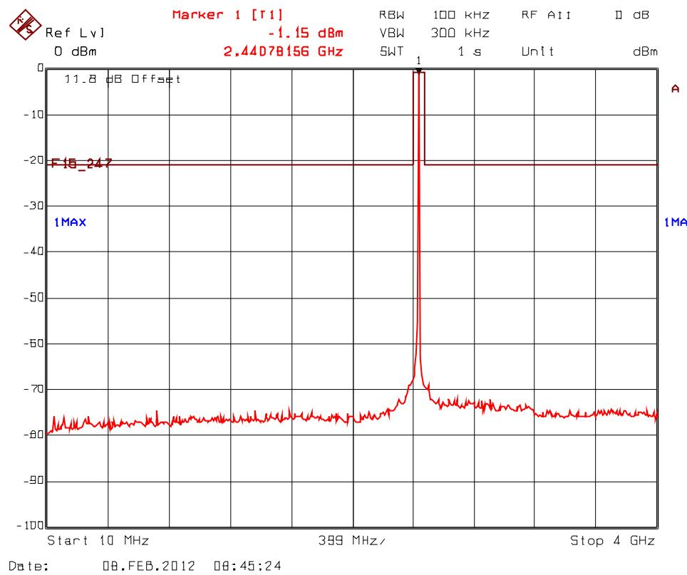
**Plot 5.9.4.2.4. Spurious RF Conducted Emissions into Non-Restricted Bands, Transceiver 1**
