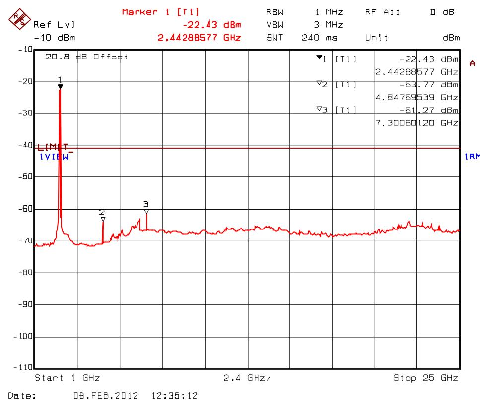
**Plot 5.9.4.3.9.** Spurious RF Conducted Emissions into Restricted Bands, Transceiver 1
