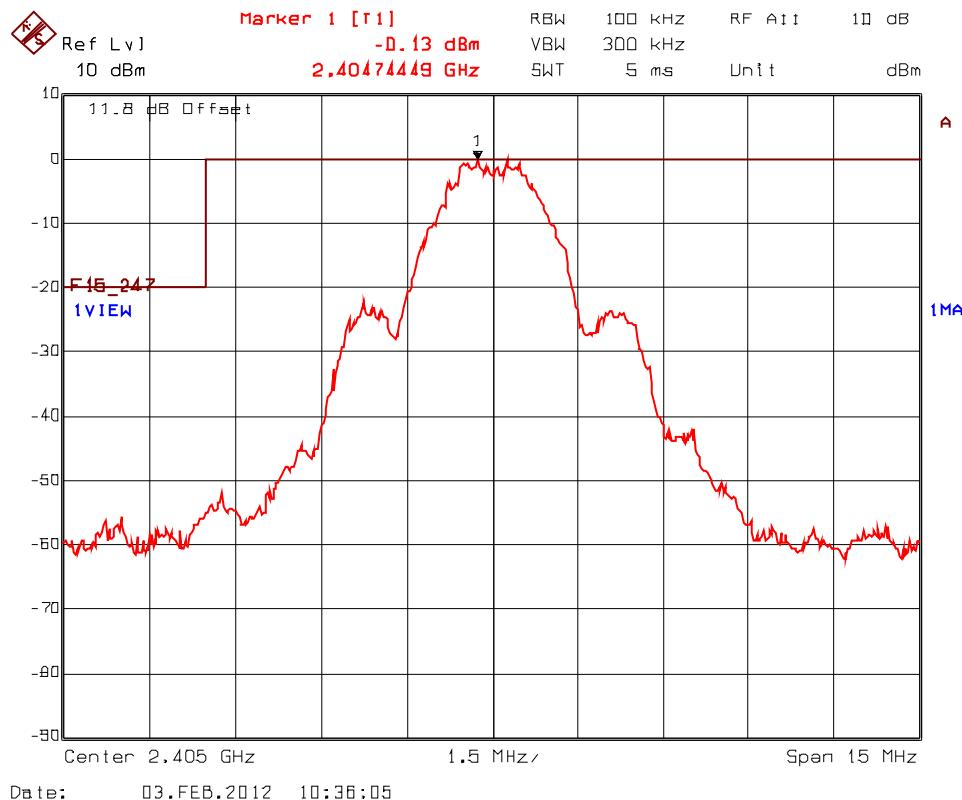
**Plot 5.9.4.1.2.** Band-Edge RF Conducted Emissions, Transceiver 1
