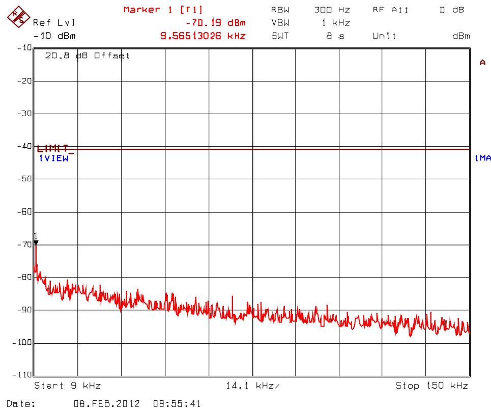
**Plot 5.9.4.3.2.** Spurious RF Conducted Emissions into Restricted Bands, Transceiver 1
