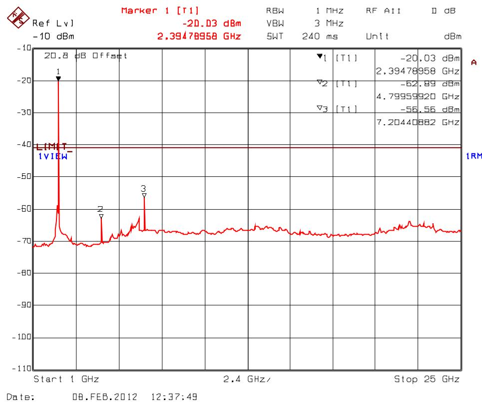
**Plot 5.9.4.3.5.** Spurious RF Conducted Emissions into Restricted Bands, Transceiver 1
