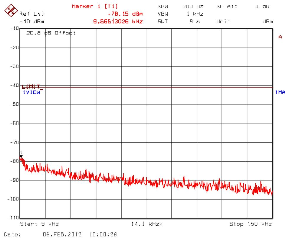
**Plot 5.9.4.3.6.** Spurious RF Conducted Emissions into Restricted Bands, Transceiver 1
