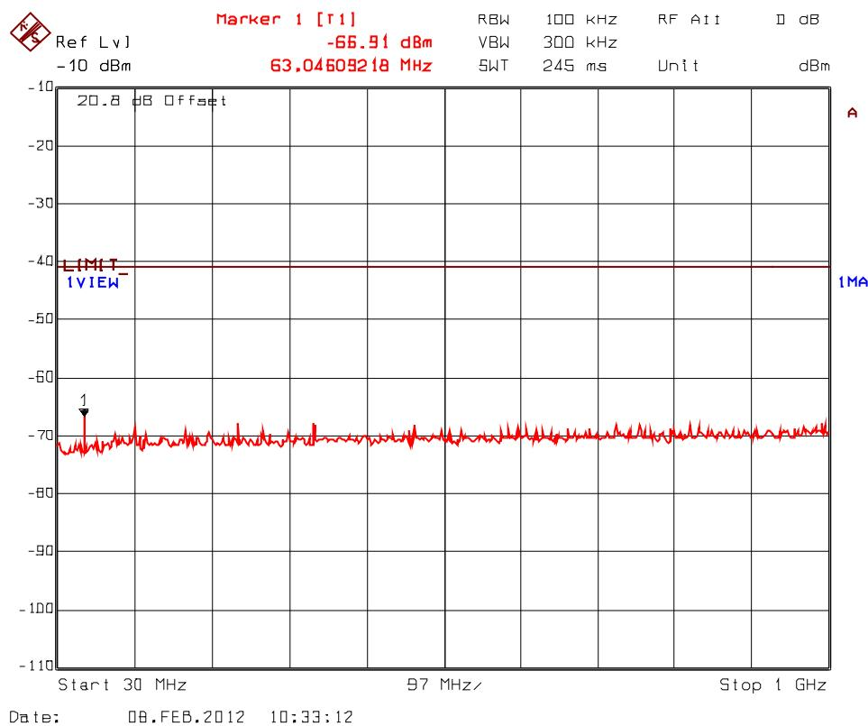
**Plot 5.9.4.3.4.** Spurious RF Conducted Emissions into Restricted Bands, Transceiver 1
