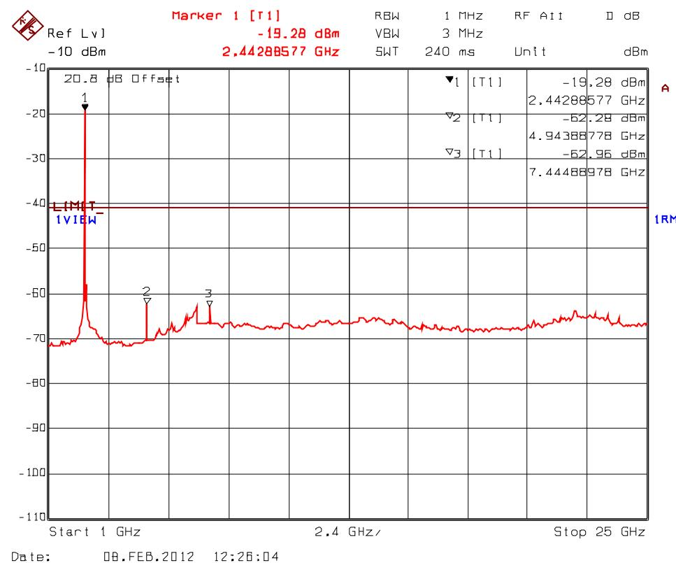
**Plot 5.9.4.3.13.** Spurious RF Conducted Emissions into Restricted Bands, Transceiver 2
