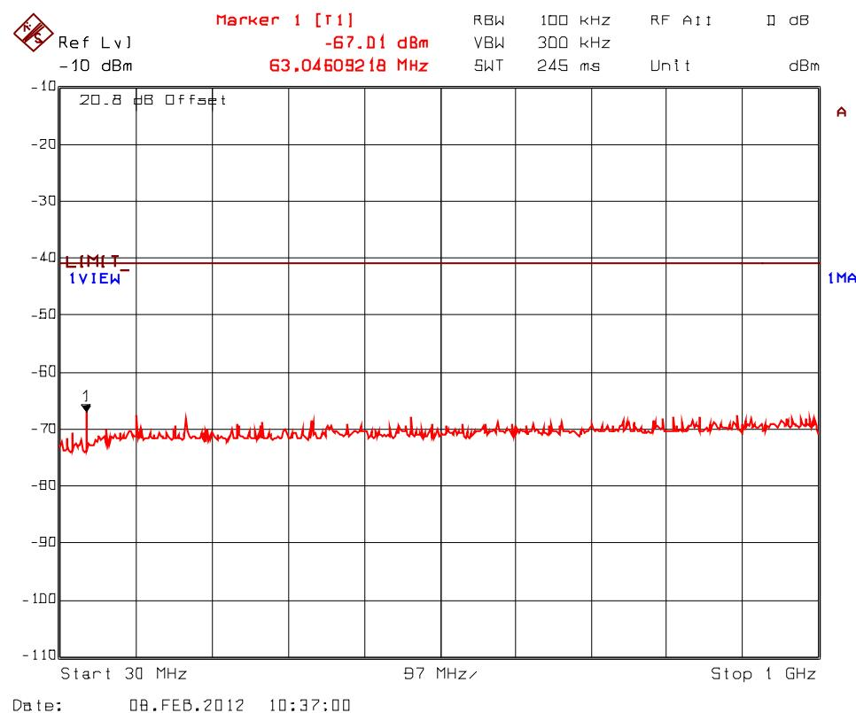
**Plot 5.9.4.3.12.** Spurious RF Conducted Emissions into Restricted Bands, Transceiver 1
