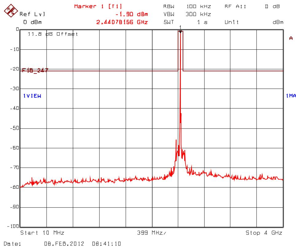
**Plot 5.9.4.2.10.** Spurious RF Conducted Emissions into Non-Restricted Bands, Transceiver 2
