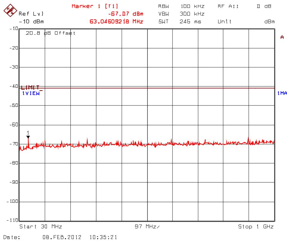
**Plot 5.9.4.3.8.** Spurious RF Conducted Emissions into Restricted Bands, Transceiver 1
