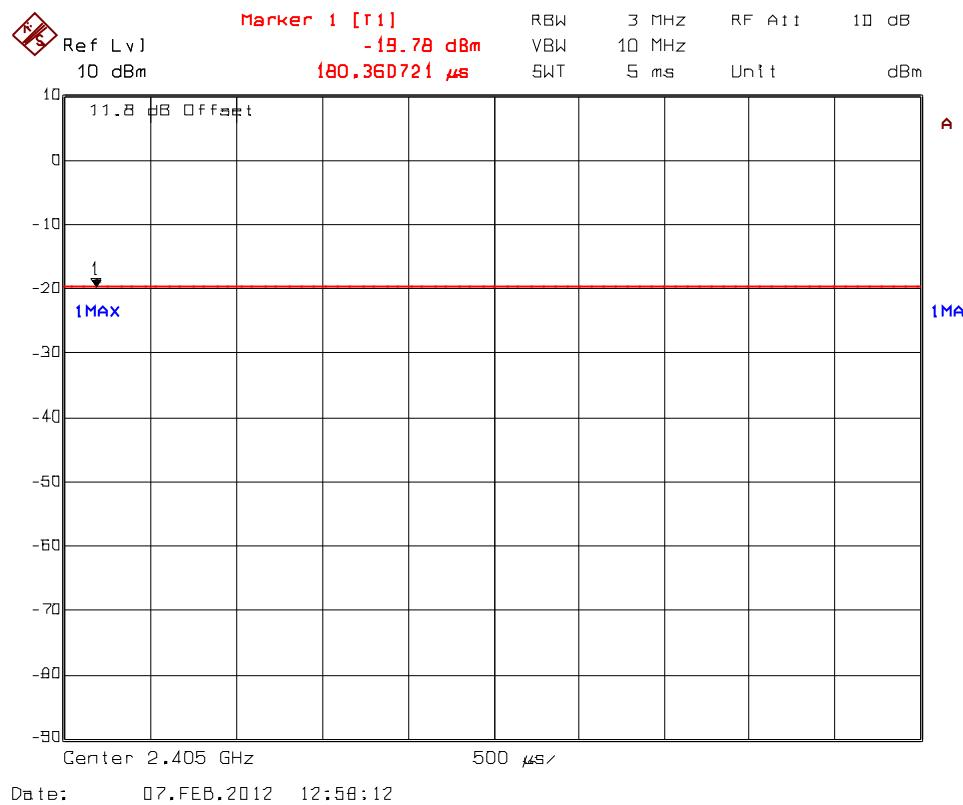
**Plot 5.8.4.8.** Maximum Peak Conducted Output Power, Low Power Setting
