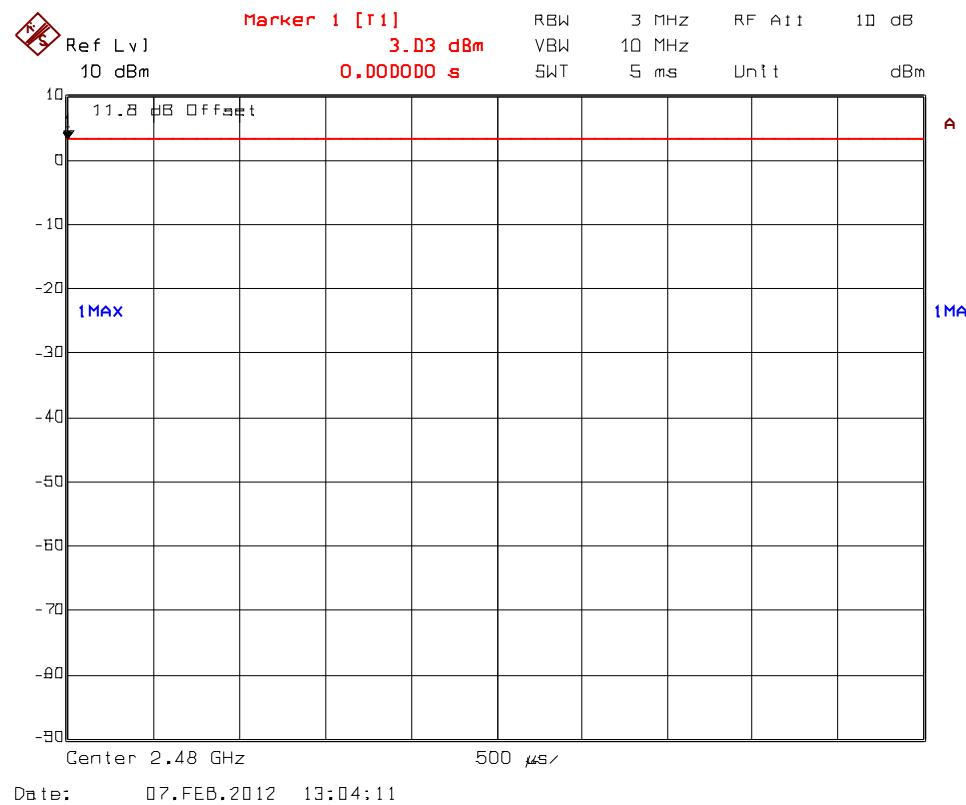
**Plot 5.8.4.7.** Maximum Peak Conducted Output Power, Low Power Setting
