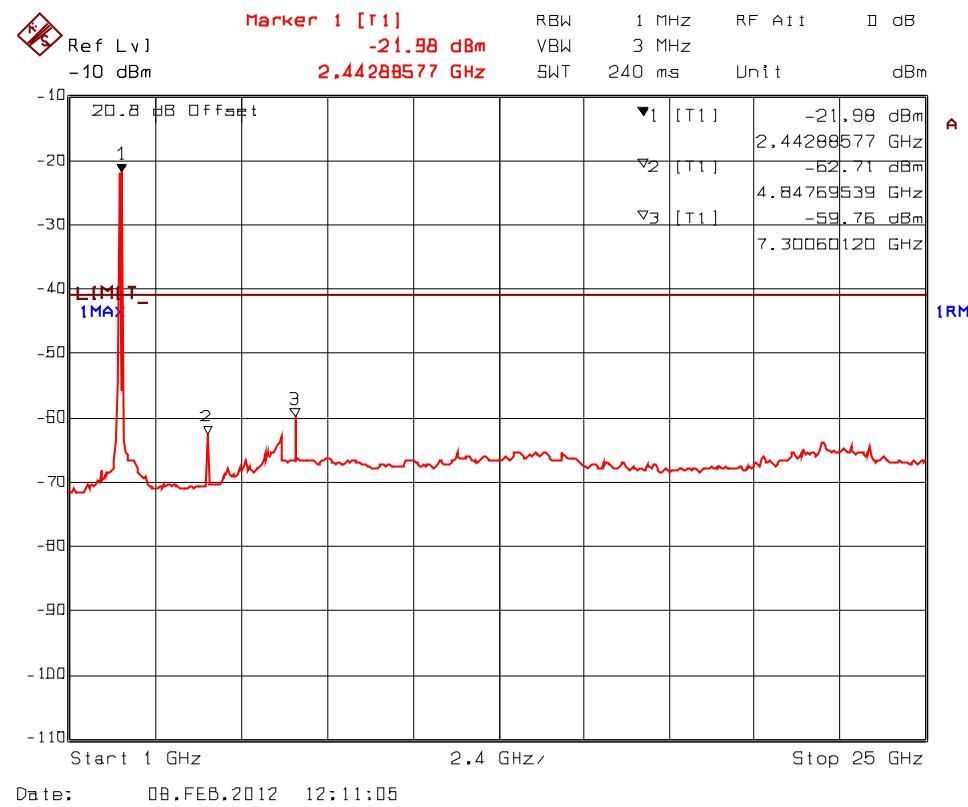
**Plot 5.9.4.3.21. Spurious RF Conducted Emissions into Restricted Bands, Transceiver 2
