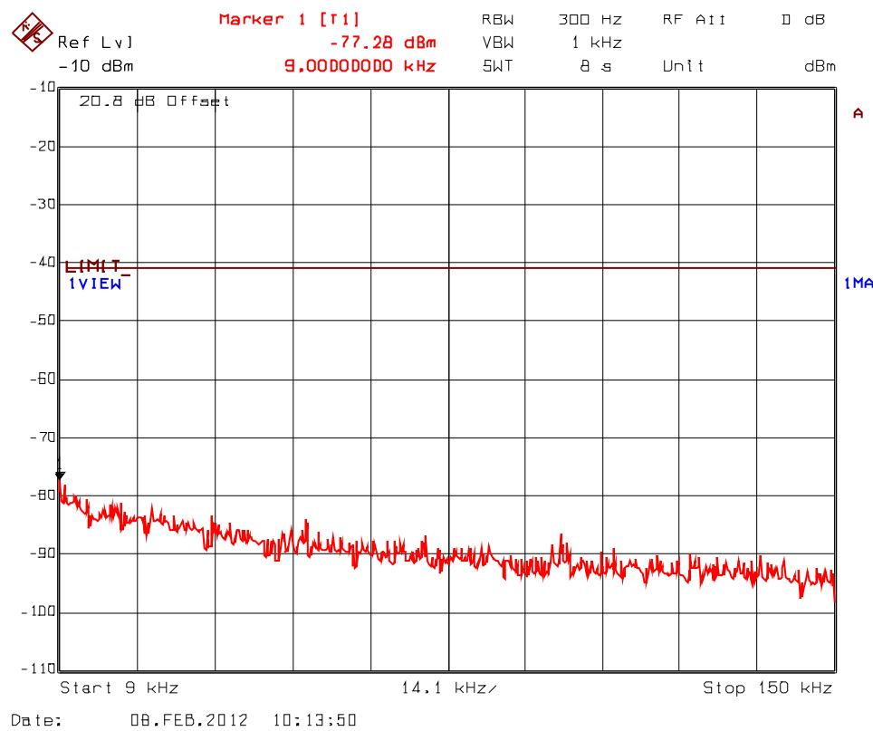
**Plot 5.9.4.3.18.** Spurious RF Conducted Emissions into Restricted Bands, Transceiver 2
