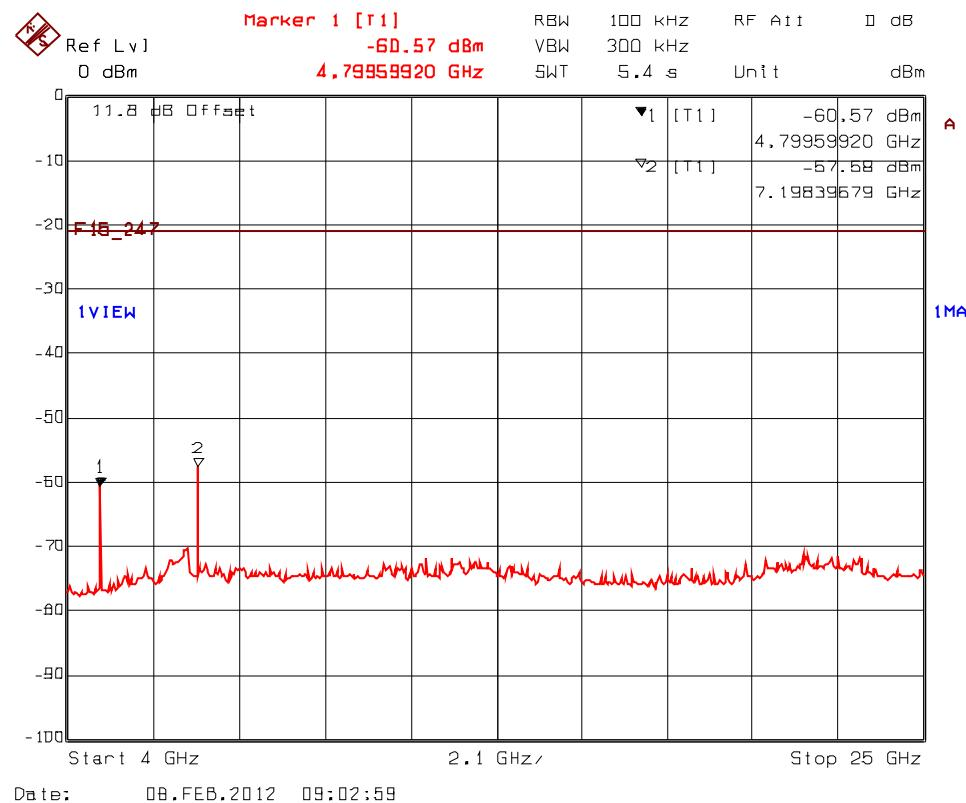
**Plot 5.9.4.2.9.** Spurious RF Conducted Emissions into Non-Restricted Bands, Transceiver 2
