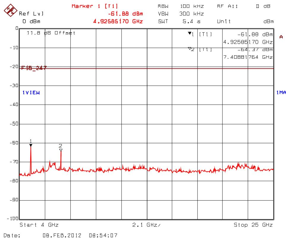
**Plot 5.9.4.2.7.** Spurious RF Conducted Emissions into Non-Restricted Bands, Transceiver 2
