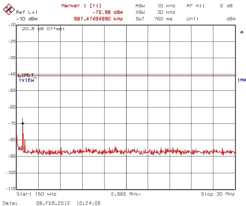
**Plot 5.9.4.3.23.** Spurious RF Conducted Emissions into Restricted Bands, Transceiver 2
