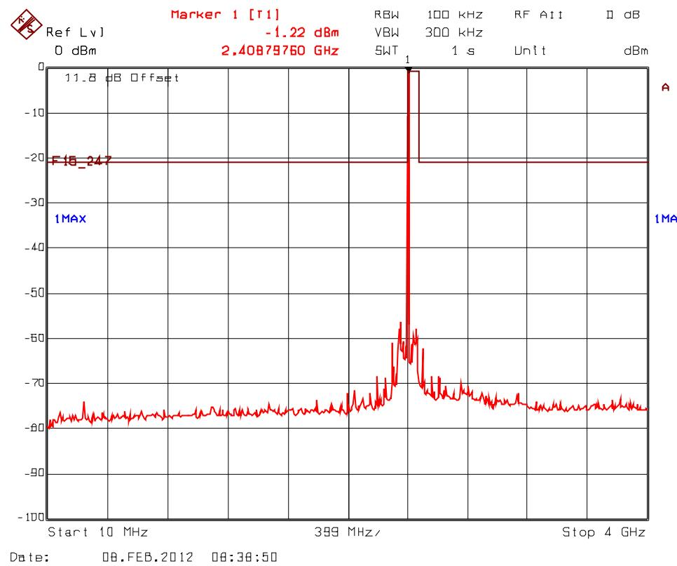
**Plot 5.9.4.2.8.** Spurious RF Conducted Emissions into Non-Restricted Bands, Transceiver 2
