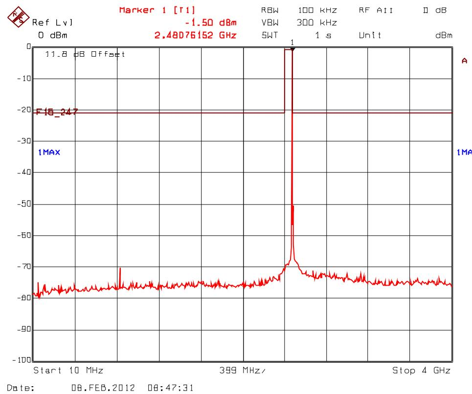
**Plot 5.9.4.2.6.** Spurious RF Conducted Emissions into Non-Restricted Bands, Transceiver 1
