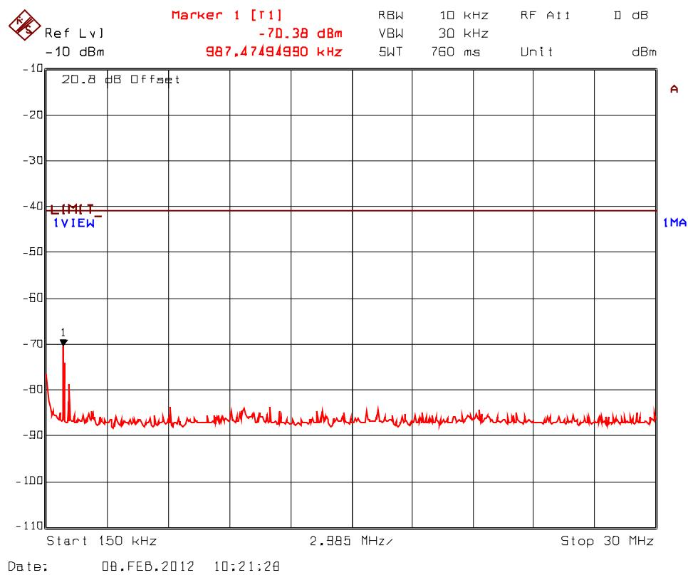
**Plot 5.9.4.3.19.** Spurious RF Conducted Emissions into Restricted Bands, Transceiver 2
