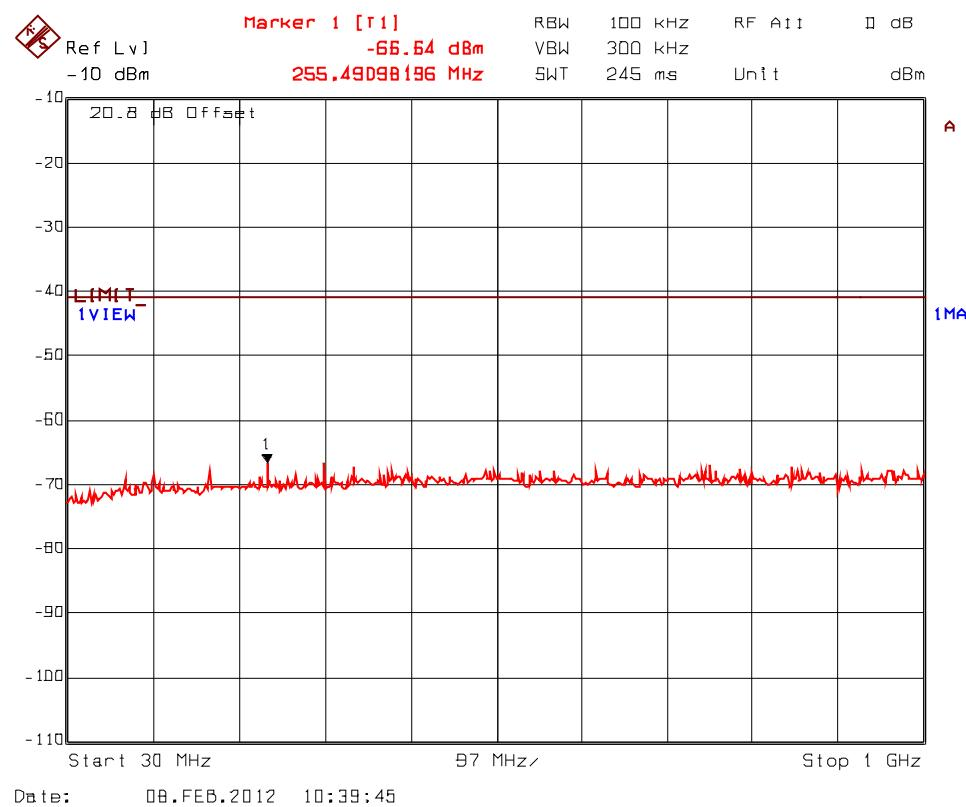
**Plot 5.9.4.3.24.** Spurious RF Conducted Emissions into Restricted Bands, Transceiver 2
