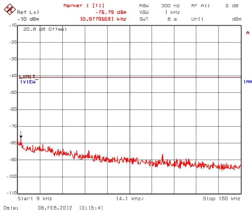
**Plot 5.9.4.3.14. Spurious RF Conducted Emissions into Restricted Bands, Transceiver 2
