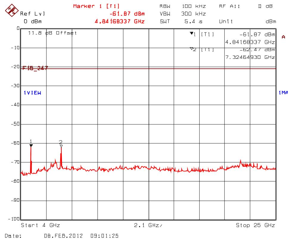
**Plot 5.9.4.2.11.** Spurious RF Conducted Emissions into Non-Restricted Bands, Transceiver 2
