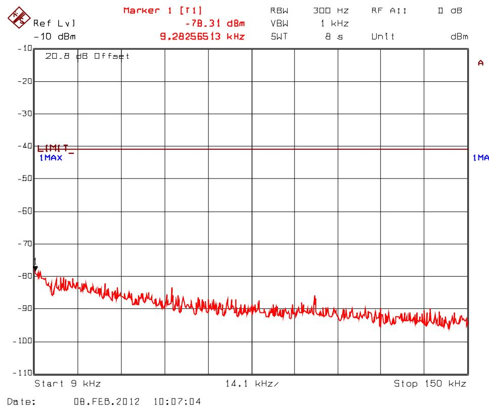
**Plot 5.9.4.3.10.** Spurious RF Conducted Emissions into Restricted Bands, Transceiver 1
