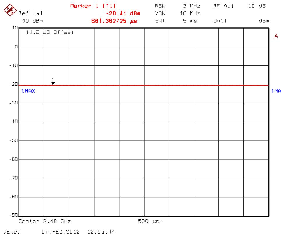
**Plot 5.8.4.10. Maximum Peak Conducted Output Power, Low Power Setting**
