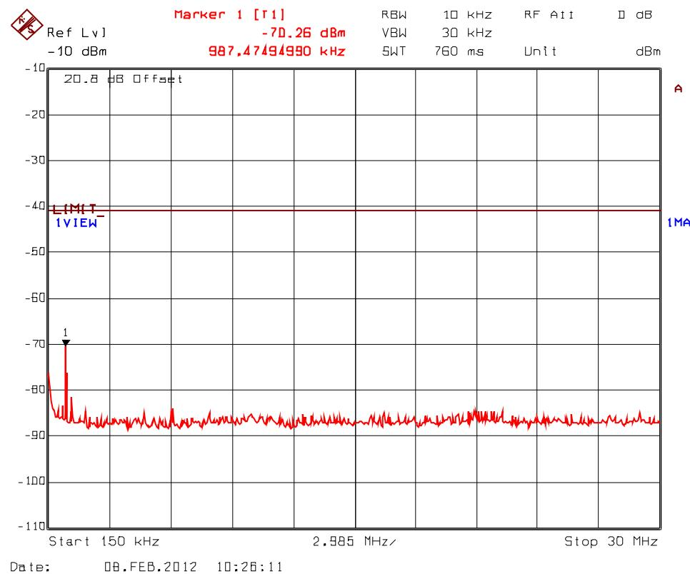
**Plot 5.9.4.3.11.** Spurious RF Conducted Emissions into Restricted Bands, Transceiver 1
