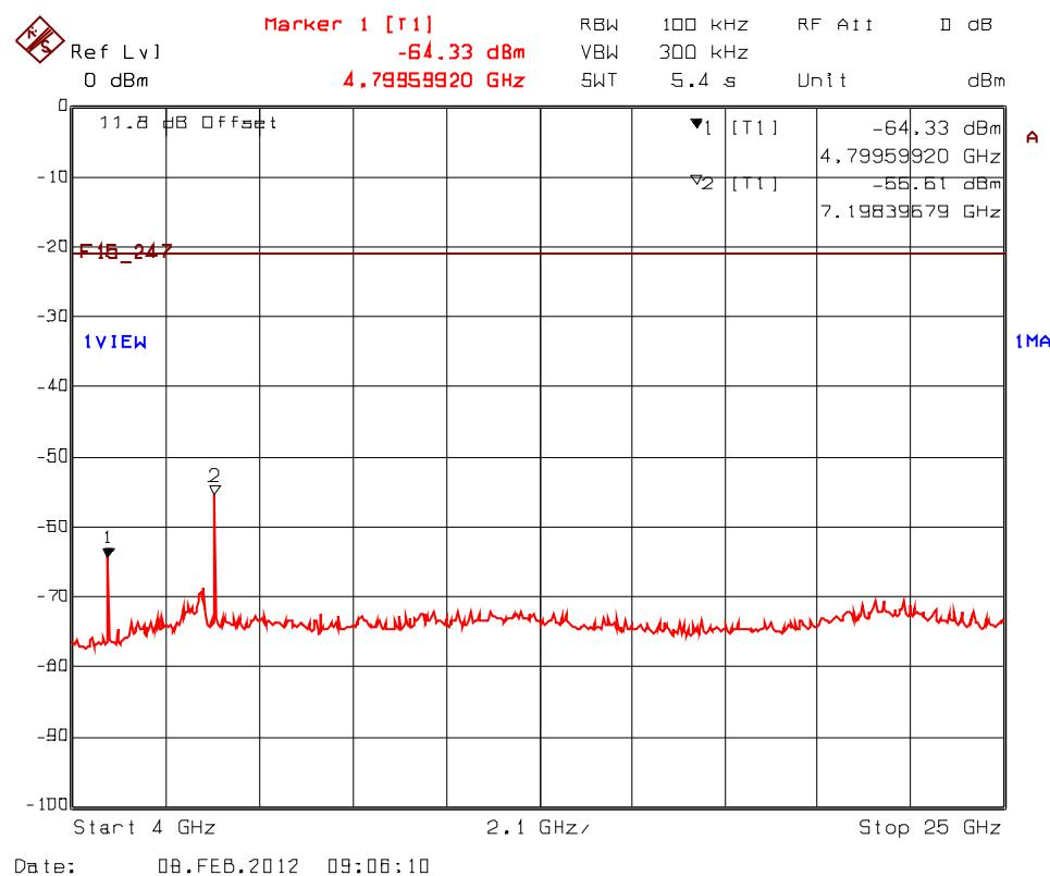
**Plot 5.9.4.2.3.** Spurious RF Conducted Emissions into Non-Restricted Bands, Transceiver 1
