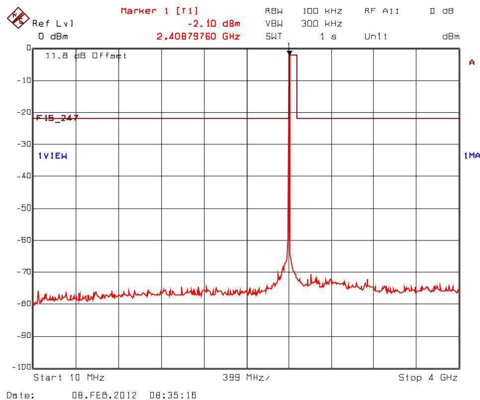
**Plot 5.9.4.2.2. Spurious RF Conducted Emissions into Non-Restricted Bands, Transceiver 1
