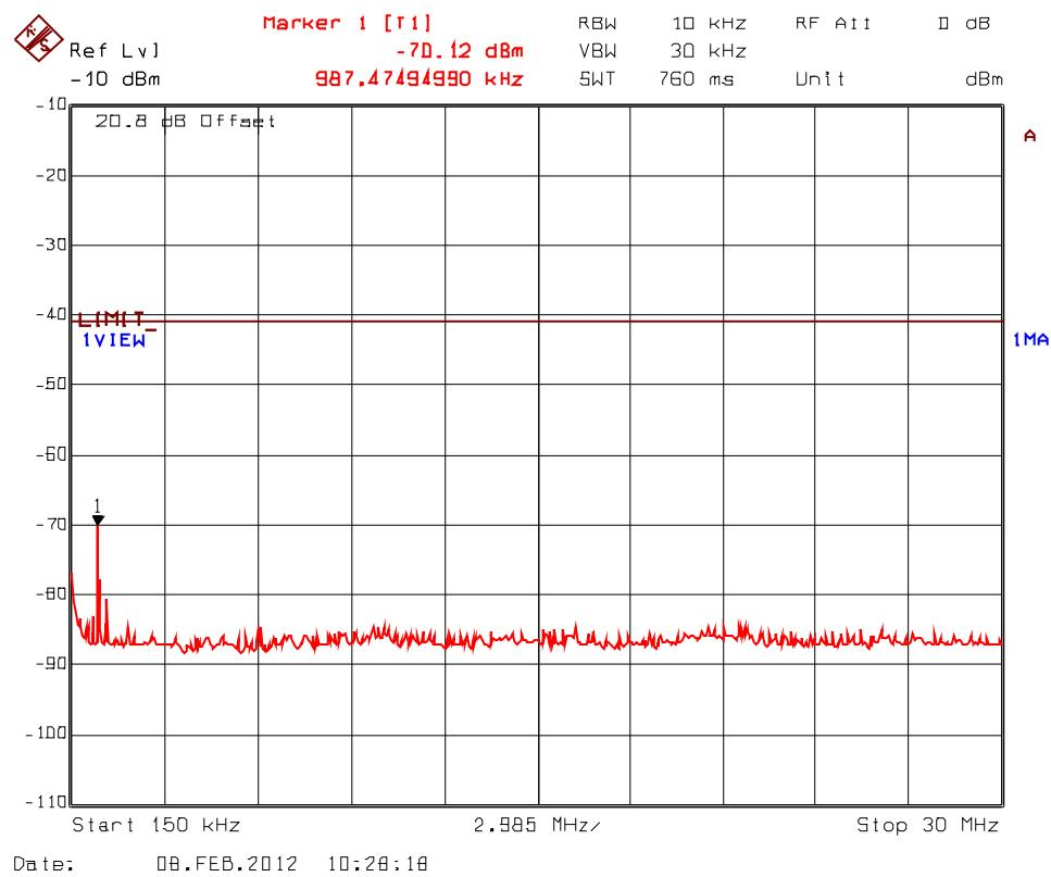
**Plot 5.9.4.3.7.** Spurious RF Conducted Emissions into Restricted Bands, Transceiver 1
