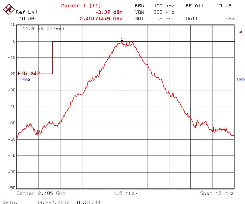
**Plot 5.9.4.1.4. Band-Edge RF Conducted Emissions, Transceiver 2
