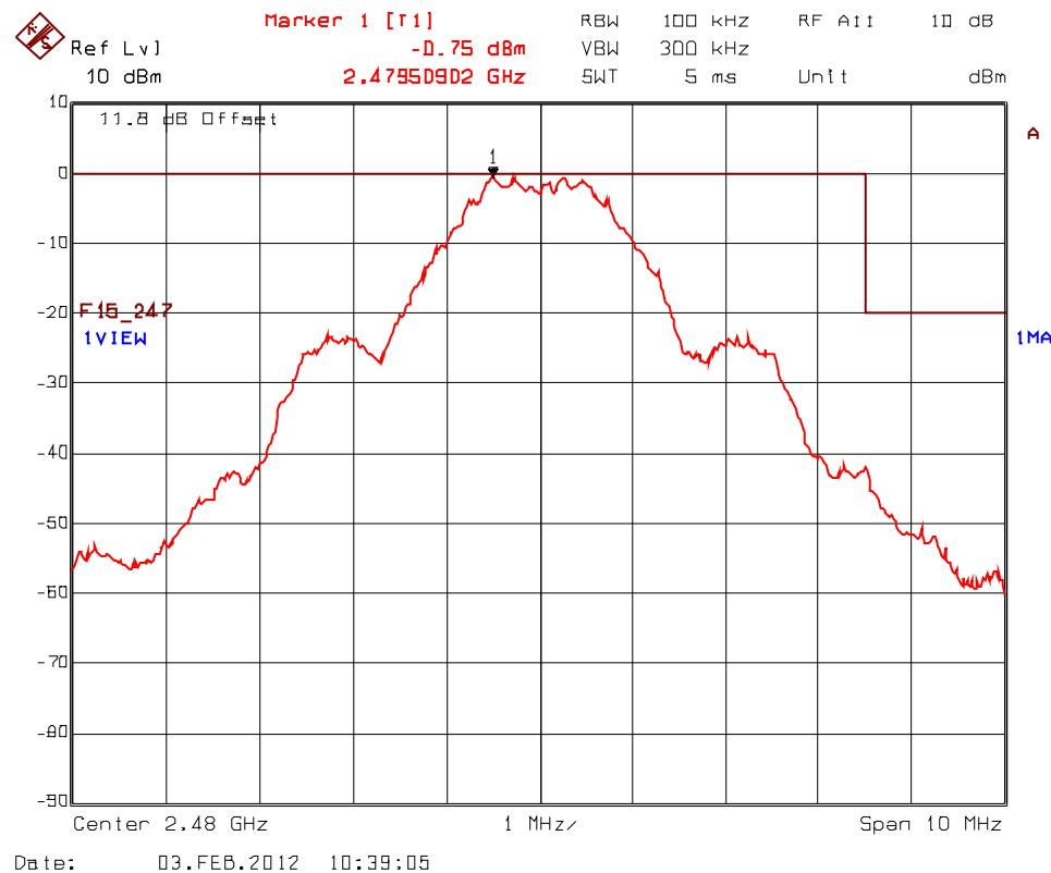
**Plot 5.9.4.1.3. Band-Edge RF Conducted Emissions, Transceiver 2
