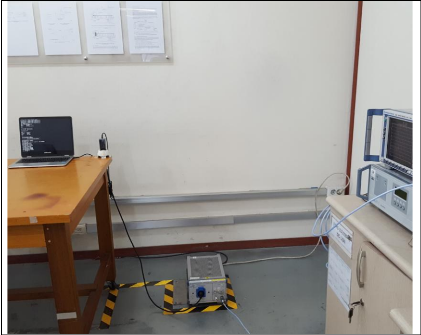
- Photo of AC Power line emission Test
