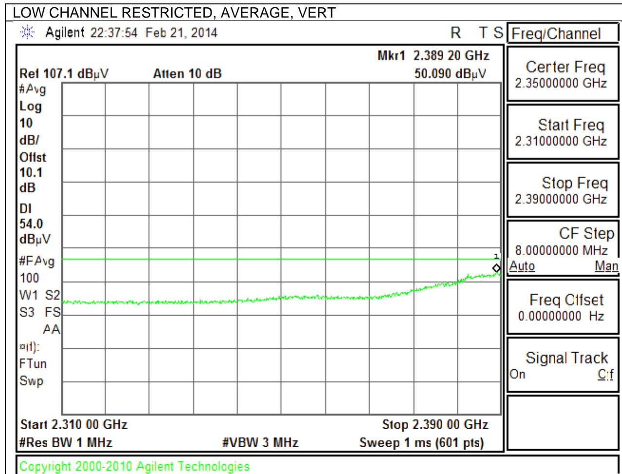
**TX ABOVE 1 GHz 802.11n HT40 CDD MODE IN THE 2.4 GHz BAND
