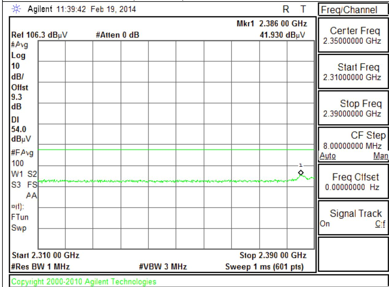
**TX ABOVE 1 GHz 802.11b MODE IN THE 2.4 GHz BAND
