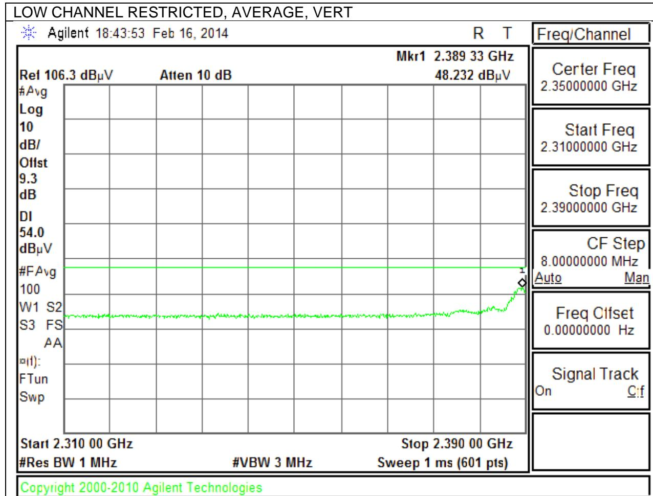
**TX ABOVE 1 GHz 802.11n HT20 MODE IN THE 2.4 GHz BAND
