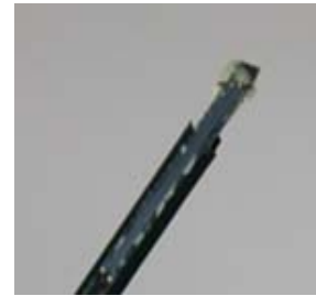
EX3DV4 E-Field Probe
