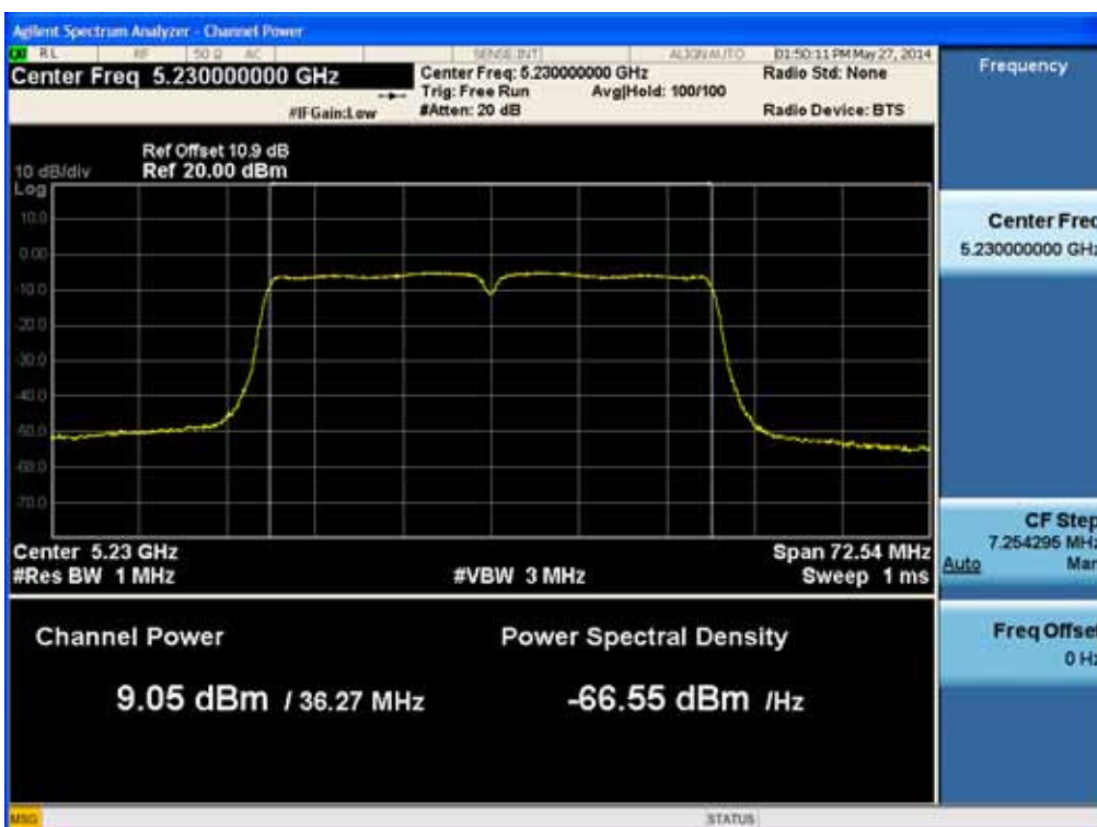
Conducted Output Power (802.11ac-CH 46) 13.5 Mbps
