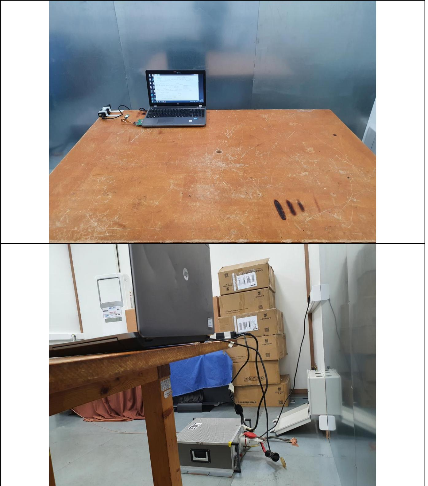
**- Radiated Emission Test (Below 1 GHz)**
